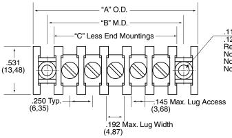
.116 Dia. Hole Both Ends .120 Recommended MTG Screws No. 2 BD. or PAN HD No. 3 MAX RD HD No. 4 MAX. FIL. HD
