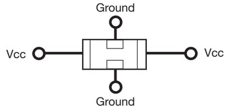
The terminals are connected internally side to side. Left side and right side are connected and front and back are connected internally. For Decoupling, the chip is usually surrounded by four vias, two for Vcc and two for GND. For Signal Filtering, the in and out lines need to be separated on the circuit board.
