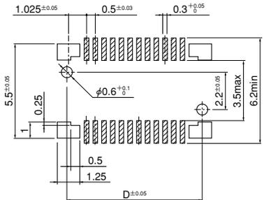
Note: 1. The above figure is the figure viewed from the connector mounting side.
