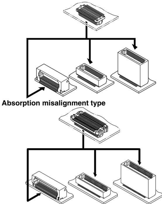
**This JMC connector is 0.5mm pitch SMT type board to board connector with selection of boss existence. Comparing with conventional JMC connector, more small and space saving are realized. Various types are available such as top/side entry type connectors including the development of the stacking height variation for plug and the absorption misalignment type for receptacle.**
