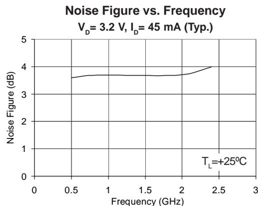
Typical RF Performance Over Temperature ( Bias:  $V_D = 3.2\text{ V}$ ,  $I_D = 45\text{ mA}$  (Typ.) )
