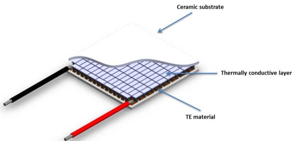
**Figure 1** Cut out of a TEM device
