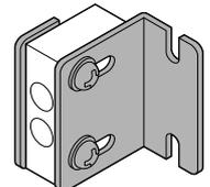
Two M3 (length 14 mm 0.551 in) screws with washers are attached.
