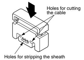
Note: The outer fluorine resin sheath of **SH-61R** cannot be peeled off with **SU-CT1**.
