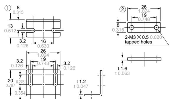
Material: Cold rolled carbon steel (SPCC) (Uni-chrome plated)
