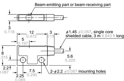
Note: The above dimensions are identical for the emitter and the receiver.
