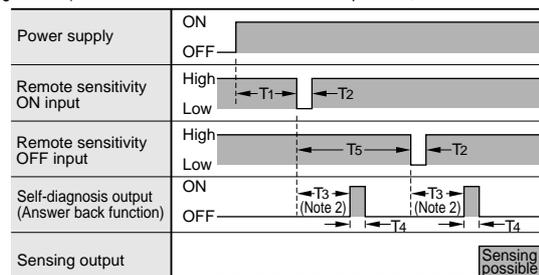
T1 ≥ 1,000 ms, 3,000 ms < T2 ≤ 5 ms, T3 ≈ 310 ms, T4 ≈ 40 ms, T5 ≥ 500 ms
