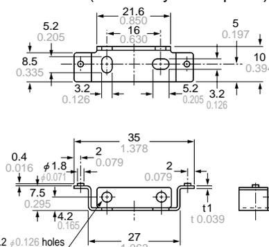
Material: Cold rolled carbon steel (SPCC)
