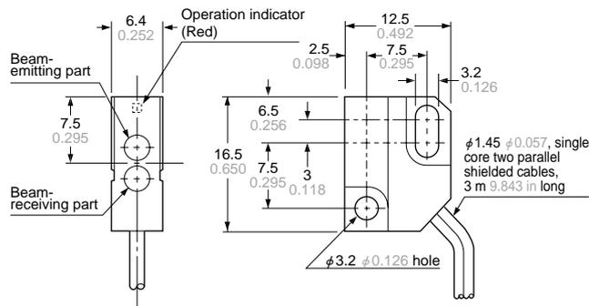
**DIMENSIONS (Unit: mm in)** The CAD data in the dimensions can be downloaded from the SUNX website: <http://www.sunx.co.jp/>
