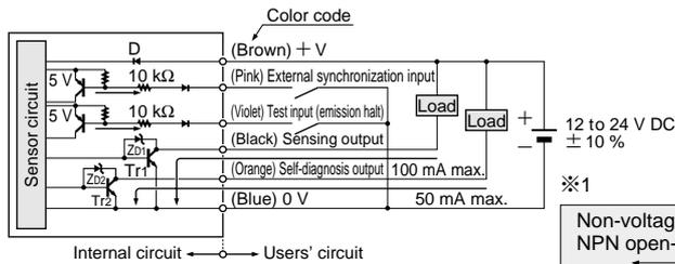
Symbols ... D: Reverse supply polarity protection diode
