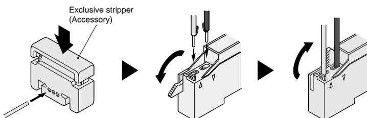
Caution: The outer fluorine sheath of the chemical resistant type sensor head, **SH-61R**, cannot be cut off with the dedicated stripper.
