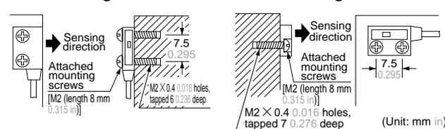
The tightening torque should be 0.14 N·m or less.
