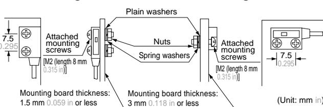
The tightening torque should be 0.14 N·m or less.
