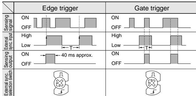
$T \geq 0.6$  ms ( $T \geq 0.8$  ms when the interference prevention function is used)
