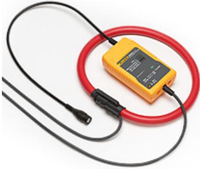
The i6000sflex is an AC current probe utilising the Rogowski principle. It can be used to measure currents up to 6000A when used in conjunction with oscilloscopes, recorders or data loggers. The flexible and lightweight measuring head allows quick and easy installation in hard to reach areas.
