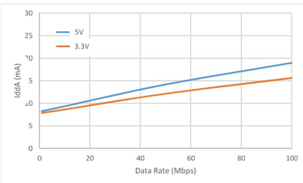
Figure 13. Si88242 Typical  $V_{DDA}$  Supply Current vs. Data Rate 5 and 3.3 V Operation
