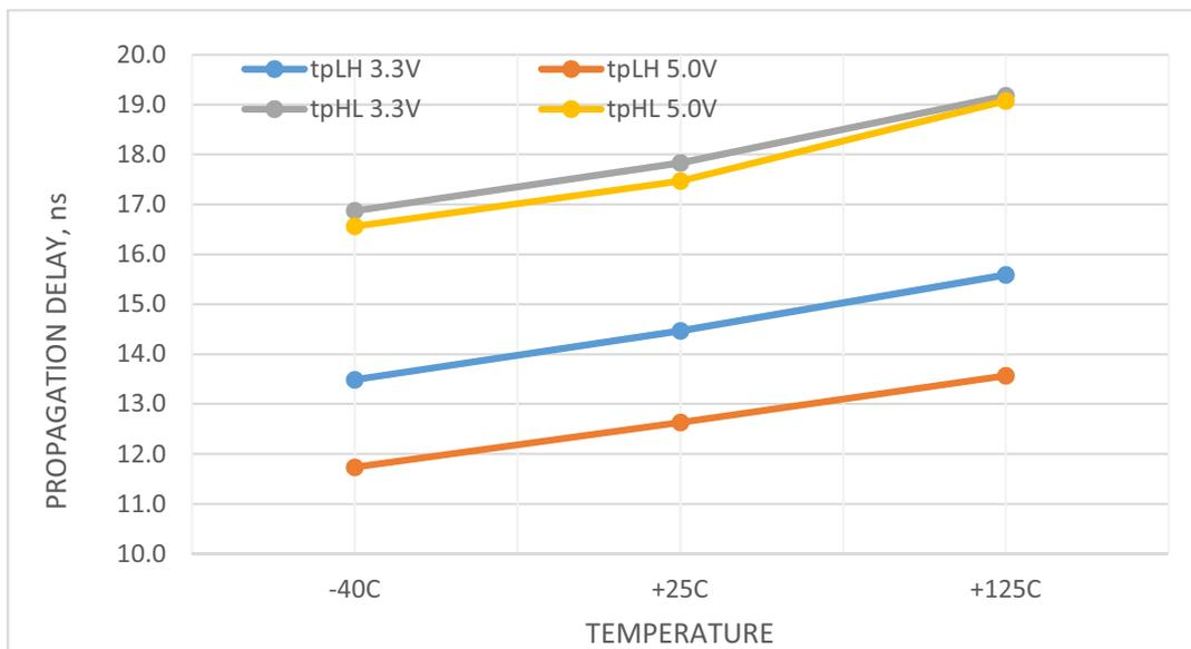
**Figure 21. Propagation Delay vs. Temperature**
