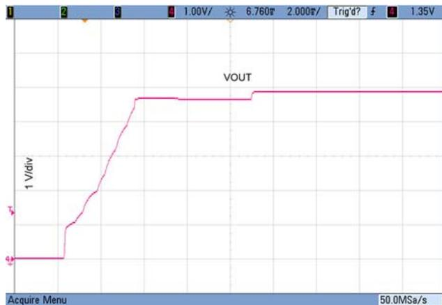
**Figure 23a. 5 V–5 V VOUT Startup vs.Time, No Load**
