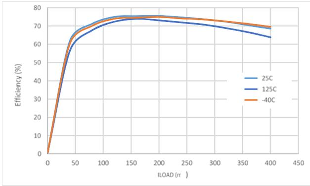
**Figure 22a. Efficiency vs. Load Current over Temperature, 3.3 V-3.3 V**
