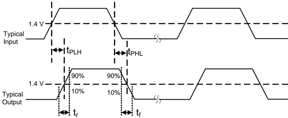
Figure 1. Propagation Delay Timing for Digital Channels
