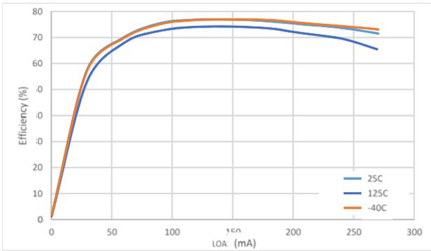
**Figure 22b. Efficiency vs. Load Current over Temperature, 3.3 V-5.0 V**
