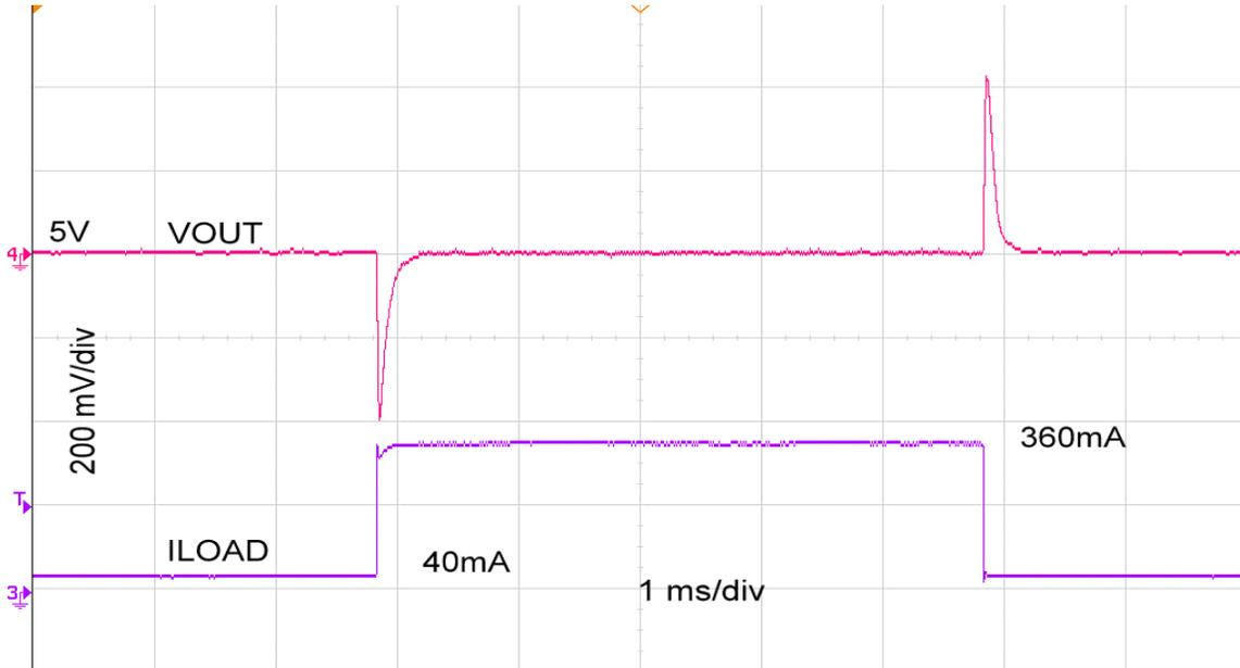
Figure 24. 5 V–5 V VOUT Load Transient Response, 10% to 90% Load
