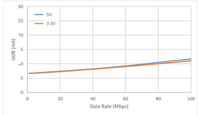
**Figure 19. Si88243 Typical  $V_{DDB}$  Supply Current vs. Data Rate 5 and 3.3 V Operation**
