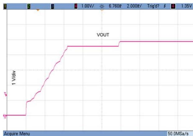
**Figure 23c. 5 V–5 V VOUT Startup vs.Time, 50 mA Load Current**
