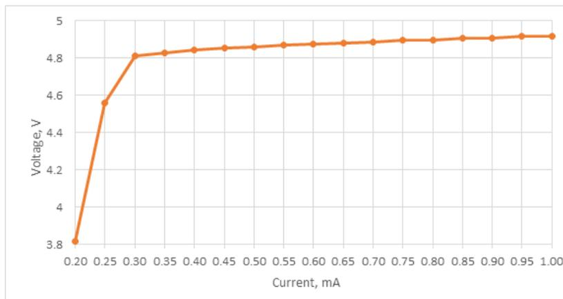
Figure 25. Typical I-V Curve for VREGA/B
