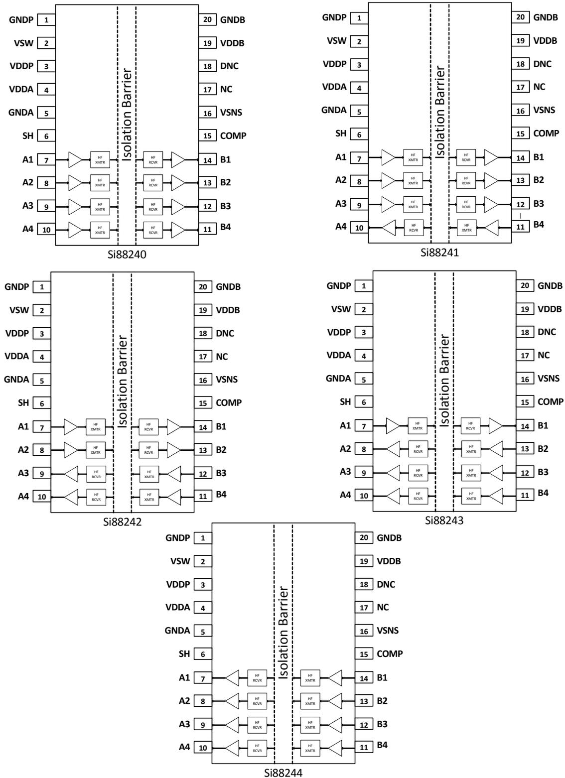
Figure 26. Si8824x Pin Configurations
