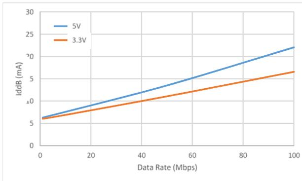
**Figure 17. Si88241 Typical  $V_{DDB}$  Supply Current vs. Data Rate 5 and 3.3 V Operation**
