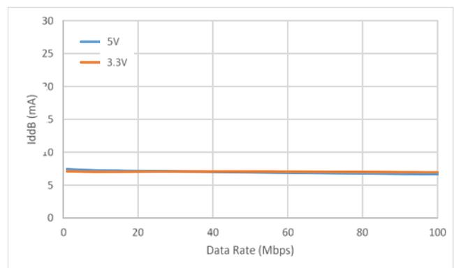
**Figure 20. Si88244 Typical  $V_{DDB}$  Supply Current vs. Data Rate 5 and 3.3 V Operation**
