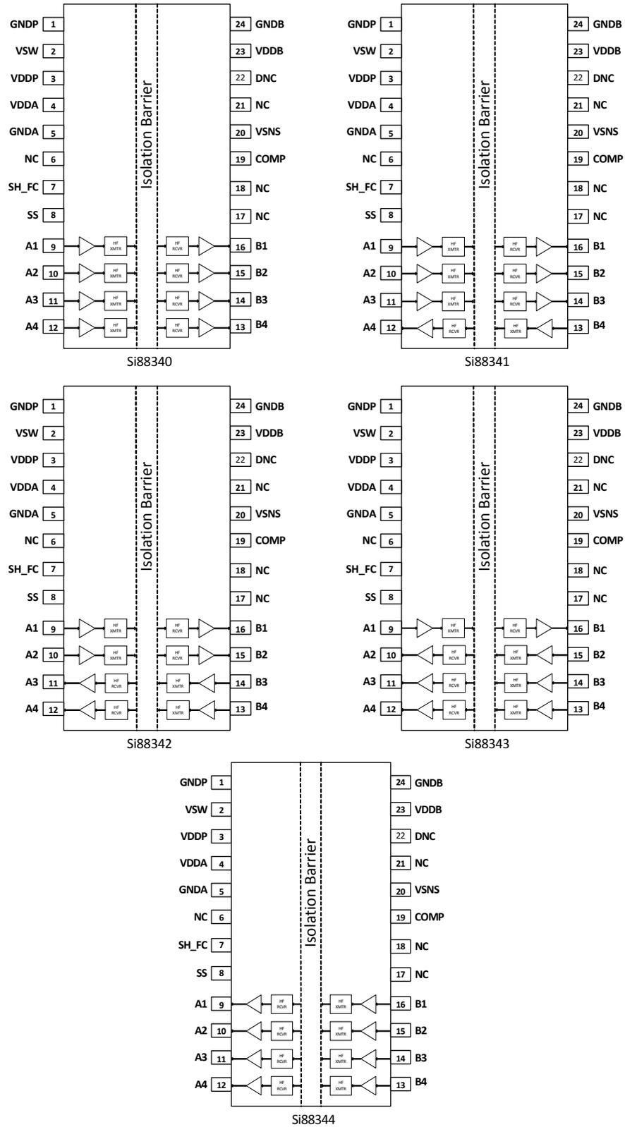
Figure 27. Si8834x Pinout Diagrams
