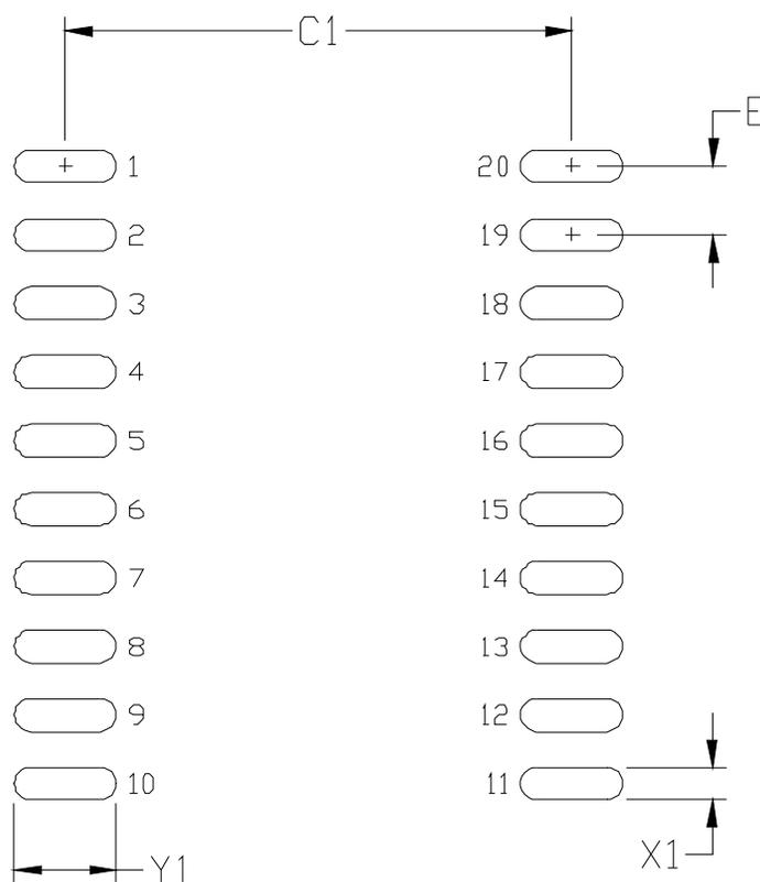
Figure 31. 20-Pin SOIC PCB Land Pattern
