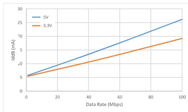
Figure 16. Si88240 Typical  $V_{DDB}$  Supply Current vs. Data Rate 5 and 3.3 V Operation
