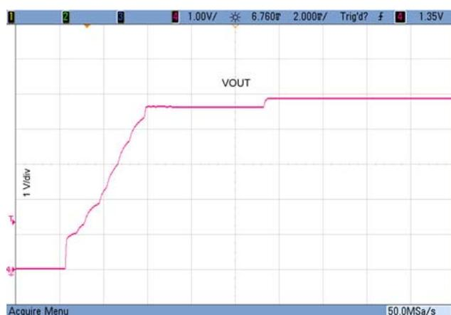
**Figure 23b. 5 V–5 V VOUT Startup vs.Time, 10 mA Load Current**
