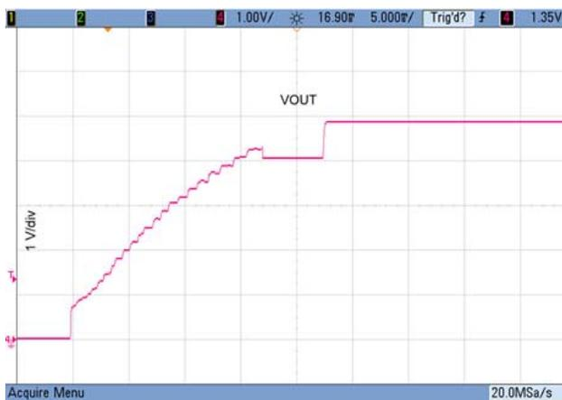
**Figure 23d. 5 V–5 V VOUT Startup vs.Time, 400 mA Load Current**
