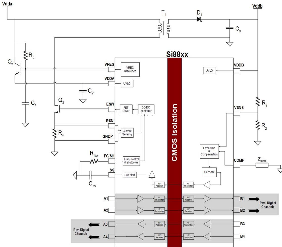
Figure 9. Si88xx Block Diagram: 24 V Input to 5 V Output
