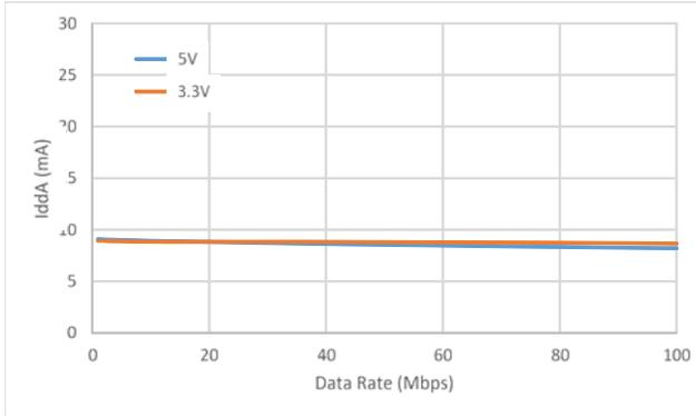
Figure 11. Si88240 Typical  $V_{DDA}$  Supply Current vs. Data Rate 5 and 3.3 V Operation
