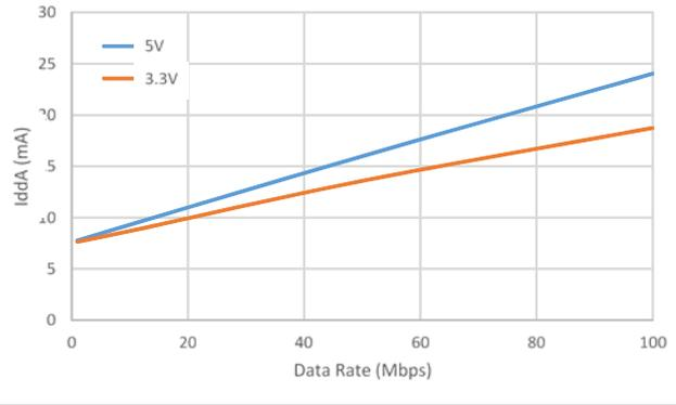
Figure 14. Si88243 Typical  $V_{DDA}$  Supply Current vs. Data Rate 5 and 3.3 V Operation
