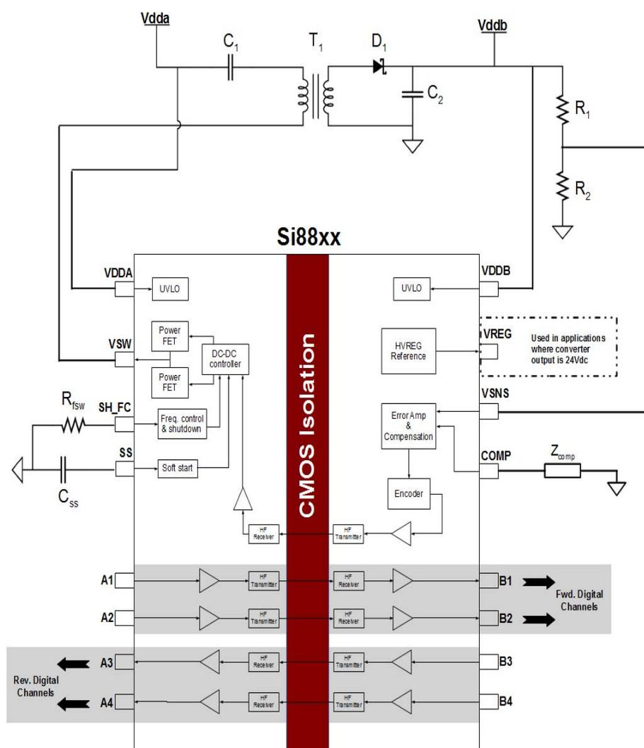
Figure 8. Si88xx Block Diagram: 3 V/3 V or 5 V/5 V Operation
