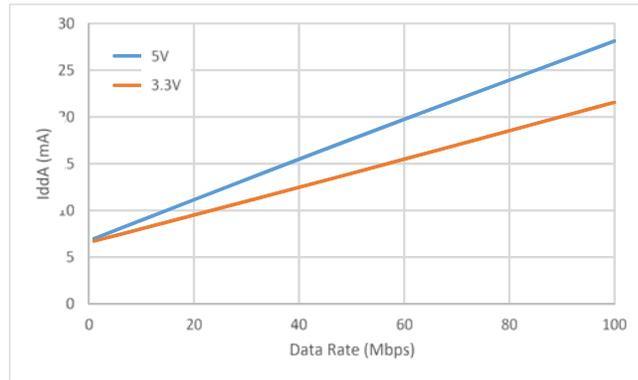
Figure 15. Si88244 Typical  $V_{DDA}$  Supply Current vs. Data Rate 5 and 3.3 V Operation
