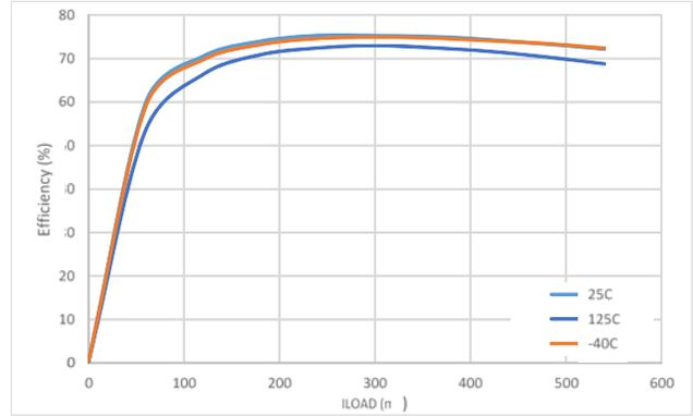
**Figure 22c. Efficiency vs. Load Current over Temperature, 5.0 V-3.3 V**
