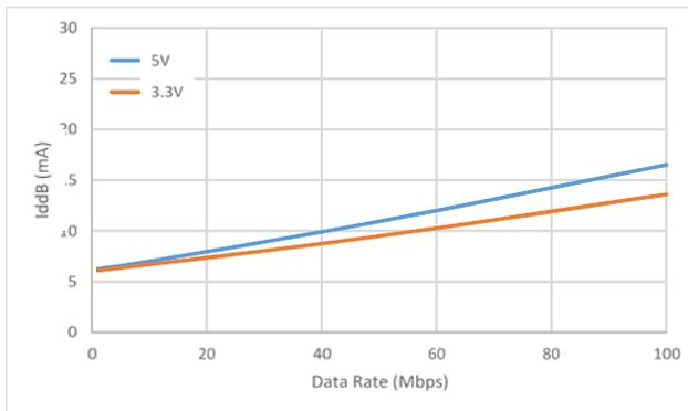
**Figure 18. Si88242 Typical  $V_{DDB}$  Supply Current vs. Data Rate 5 and 3.3 V Operation**
