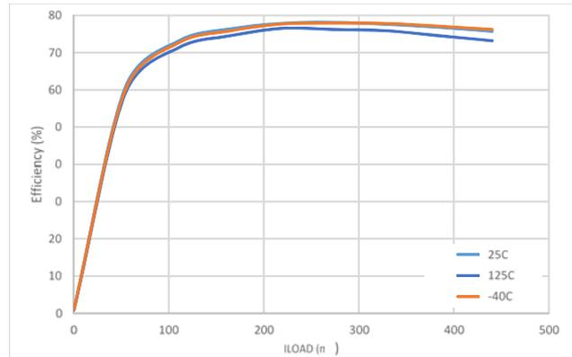
**Figure 22d. Efficiency vs. Load Current over Temperature, 5.0 V-5.0 V**
