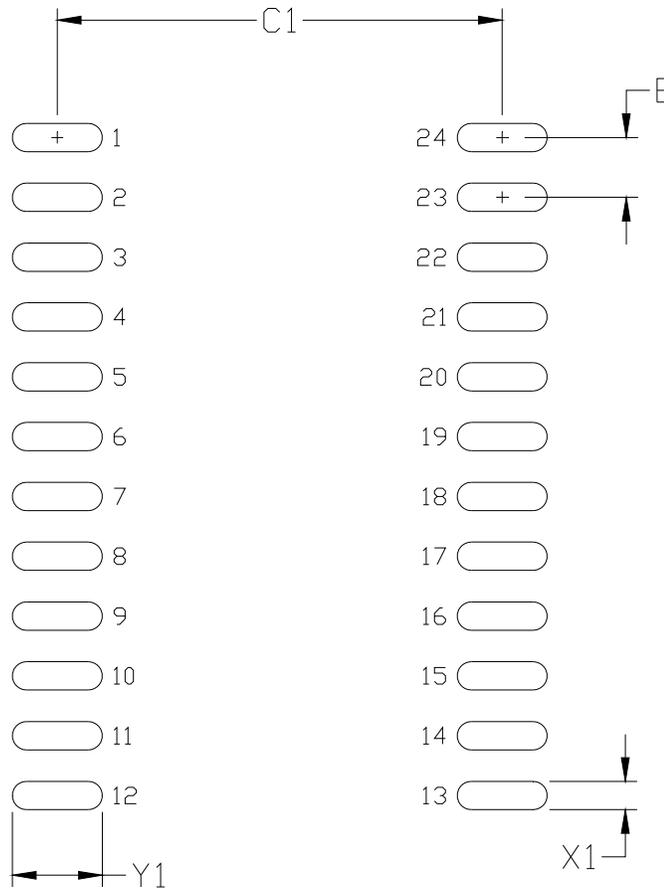
**Figure 33. 24-Pin SOIC PCB Land Pattern**
