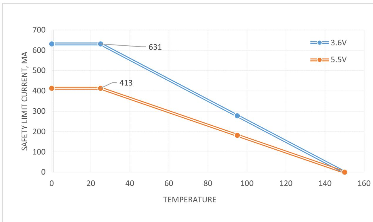
Figure 5. WB SOIC-20 Thermal Derating Curve\*
