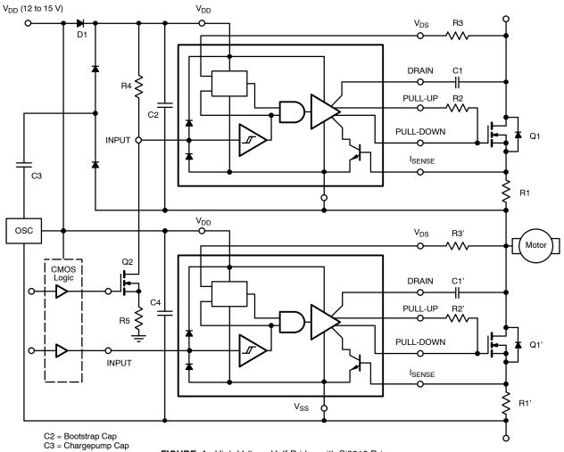
FIGURE 1. High-Voltage Half-Bridge with Si9910 Drivers
