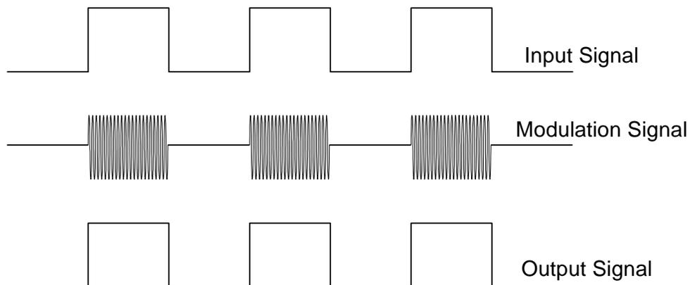
**Figure 7. Modulation Scheme**
