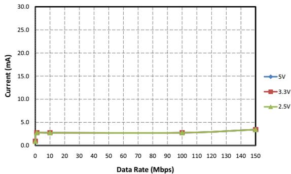
**Figure 10. Si8630/35 Typical  $V_{DD1}$  Supply Current vs. Data Rate 5, 3.3, and 2.5 V Operation**
