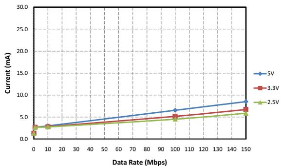
**Figure 11. Si8631 Typical  $V_{DD1}$  Supply Current vs. Data Rate 5, 3.3, and 2.5 V Operation**
