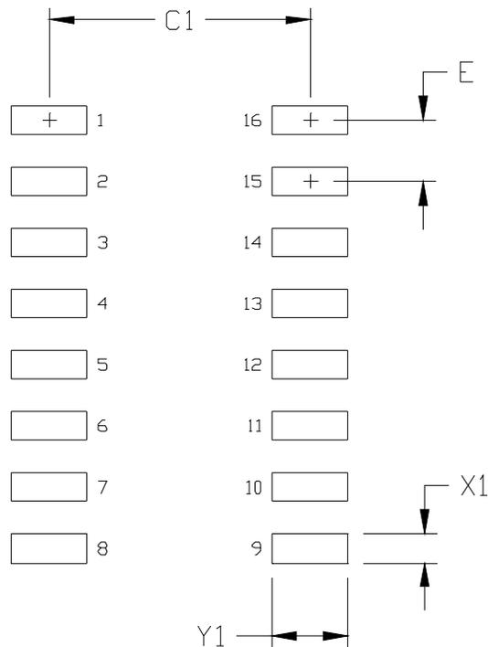
**Figure 18. 16-Pin Narrow Body SOIC PCB Land Pattern**
