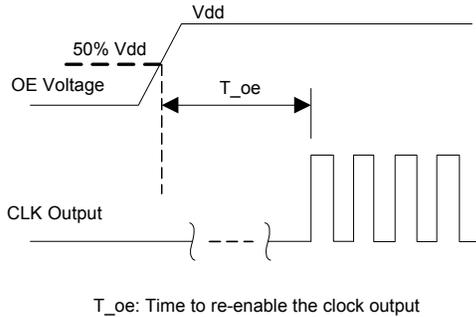
**Figure 9. OE Enable Timing (OE Mode Only)**
