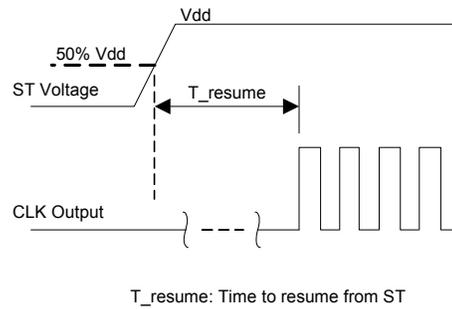
**Figure 8. Standby Resume Timing (ST Mode Only)**
