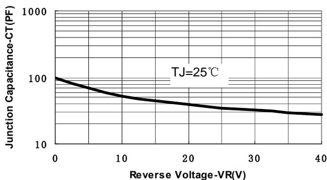
Fig.1-Typical Junction Capacitance
