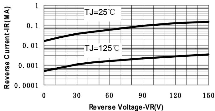
Fig.2-Typical Reverse Characteristics
