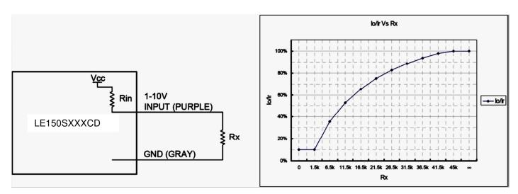
**Dimming Configuration using External Resistance**
