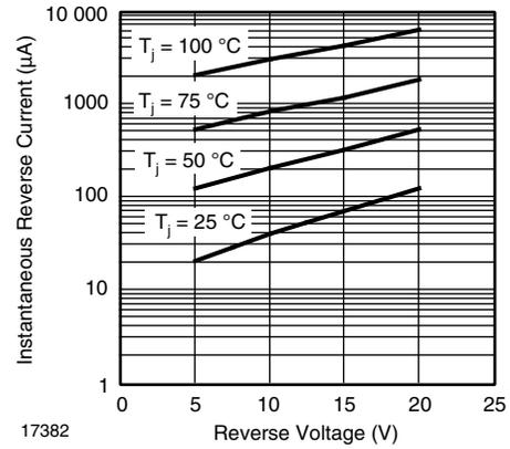
Figure 4. Typical Reverse Current Characteristics - SL02
