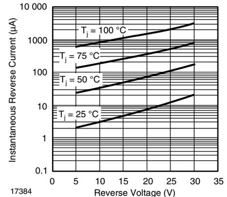
Figure 6. Typical Reverse Current Characteristics - SL03
