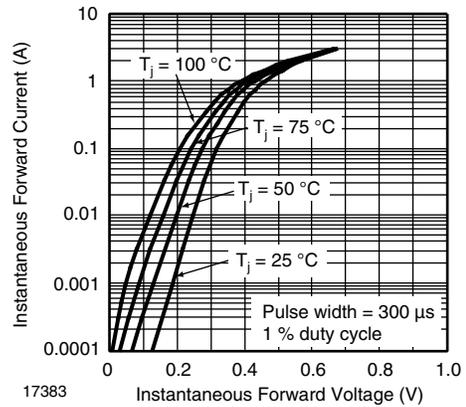
Figure 5. Typical Instantaneous Forward Characteristics - SL03
