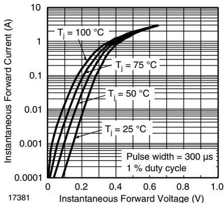
Figure 3. Typical Instantaneous Forward Characteristics - SL02
