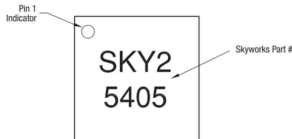
**Figure 8. Typical Part Markings**
