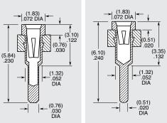
Contact Length = (2.11 mm) .083" Lead DIA Accepted = (0.38 mm) .015" to (0.51 mm) .020" Insertion Depth = (2.67 mm) .105" to (4.32 mm) .170" Style 10 Component Part No. = SC-3P1
