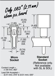
Insertion Depth = (1.65 mm) .065" to (3.56 mm) .140" Style 19 Component Part No. = SC-8P1
