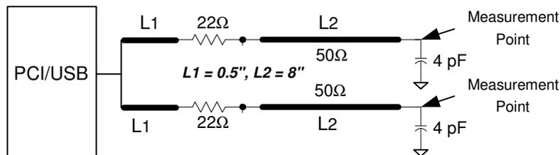
**Figure 9. Single-ended PCI and USB Double Load Configuration**
