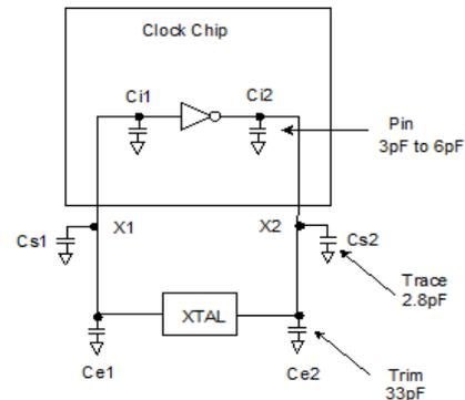
**Figure 2. Crystal Loading Example**
