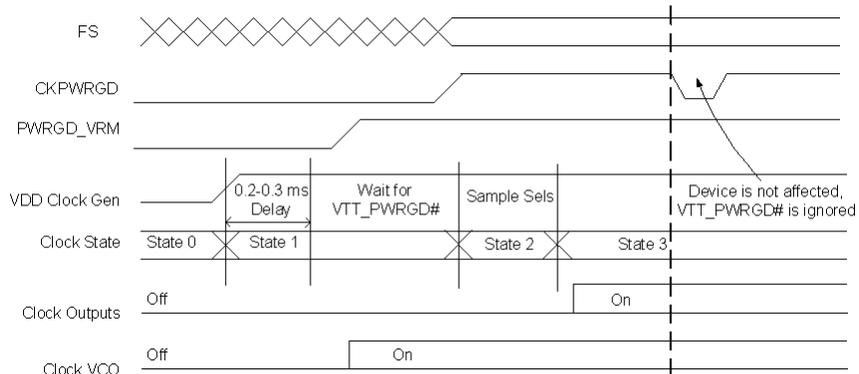
Figure 5. CKPWRGD Timing Diagram
