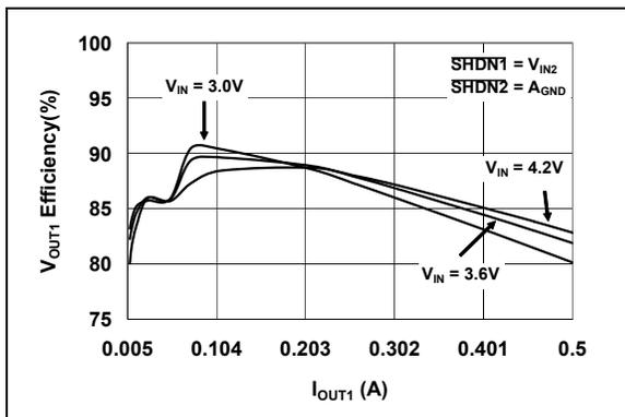
**FIGURE 2-8:**  $V_{OUT1}$  Output Efficiency vs.  $I_{OUT1}$  ( $V_{OUT1} = 1.8\text{V}$ ).
