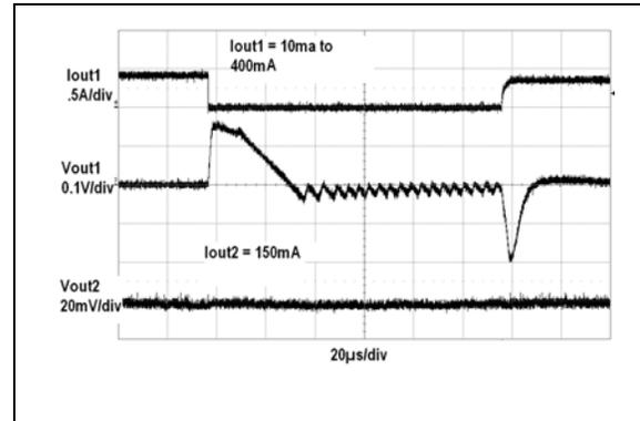
**FIGURE 2-36:**  $V_{OUT1}$  Load Step Response vs. Time.
