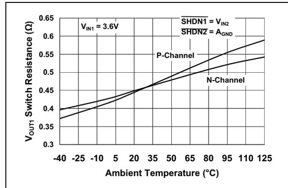
**FIGURE 2-18:**  $V_{OUT1}$  Switch Resistance vs. Ambient Temperature.
