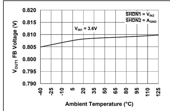
**FIGURE 2-16:**  $V_{OUT1}$  Adjustable Feedback Voltage vs. Ambient Temperature.
