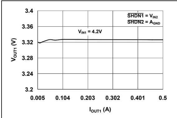
**FIGURE 2-13:**  $V_{OUT1}$  vs.  $I_{OUT1}$
