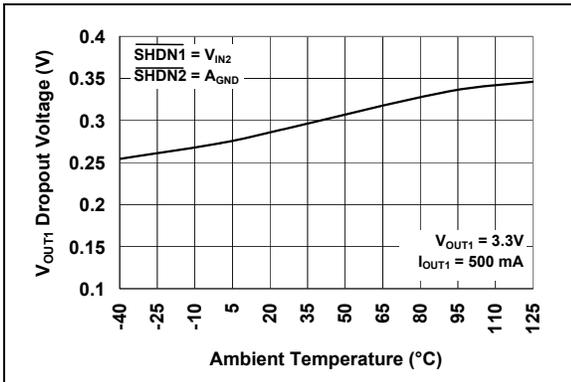
**FIGURE 2-19:**  $V_{OUT1}$  Dropout Voltage vs. Ambient Temperature.
