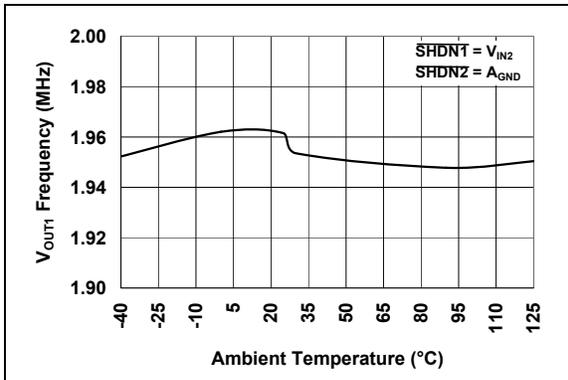
**FIGURE 2-15:**  $V_{OUT1}$  Switching Frequency vs. Ambient Temperature.
