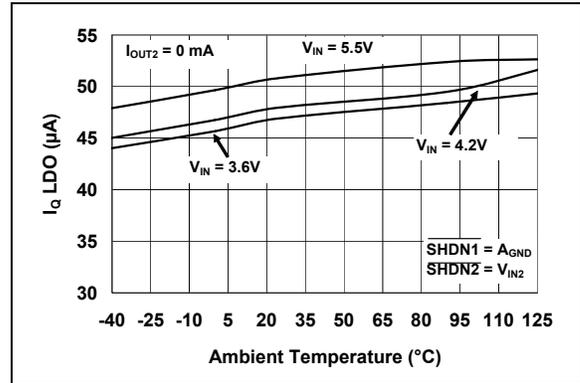
**FIGURE 2-4:**  $I_Q$  LDO Current vs. Ambient Temperature.
