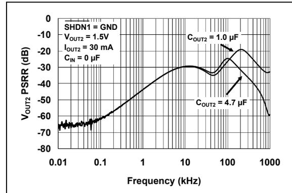
**FIGURE 2-34:**  $V_{OUT2}$  Power Supply Ripple Rejection vs. Frequency.
