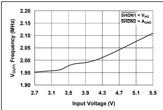
**FIGURE 2-14:**  $V_{OUT1}$  Switching Frequency vs. Input Voltage.
