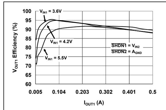
**FIGURE 2-10:**  $V_{OUT1}$  Output Efficiency vs.  $I_{OUT1}$  ( $V_{OUT1} = 3.3\text{V}$ ).
