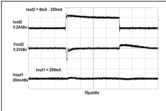
**FIGURE 2-37:**  $V_{OUT2}$  Load Step Response vs. Time.
