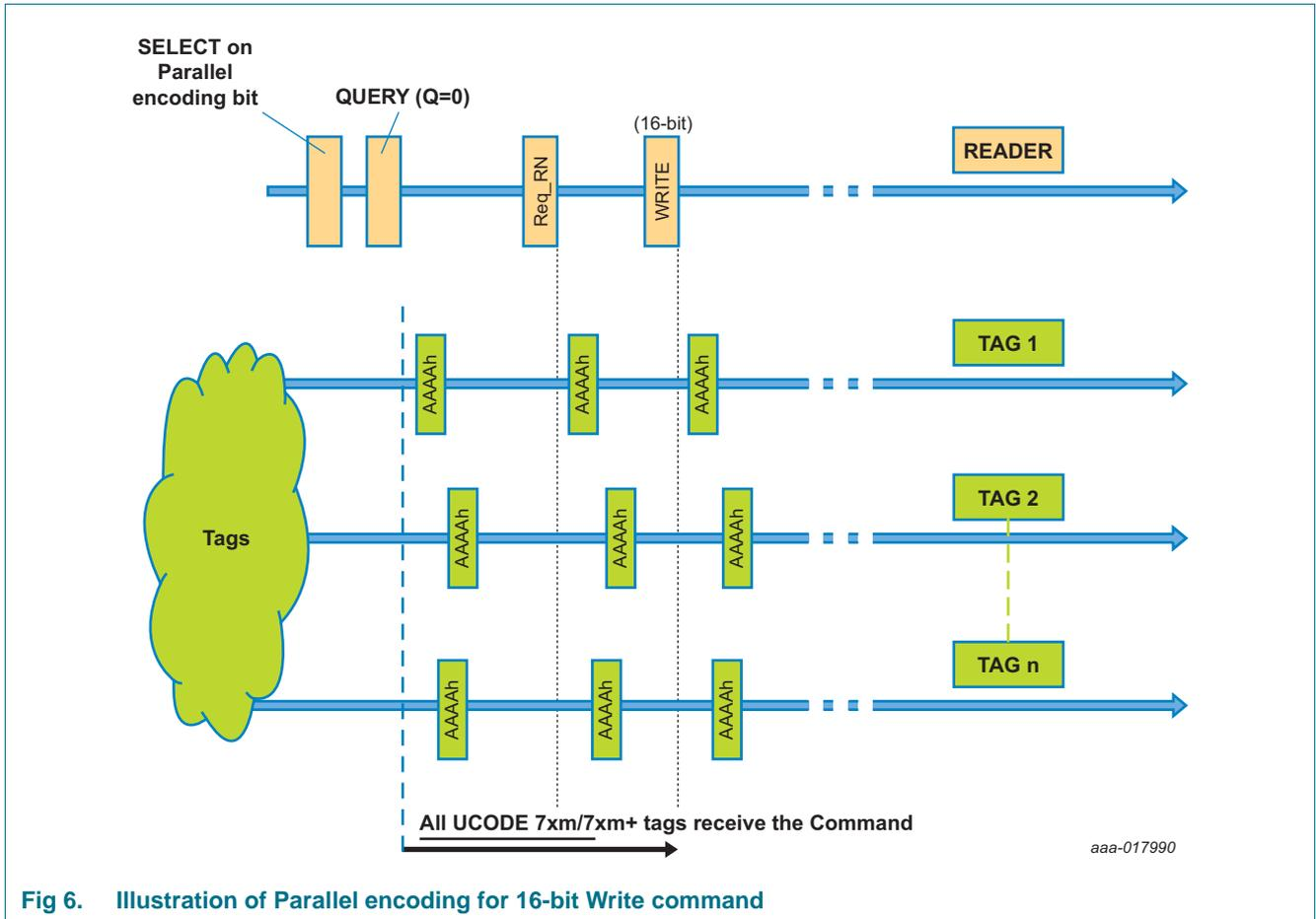
Fig 6. Illustration of Parallel encoding for 16-bit Write command
