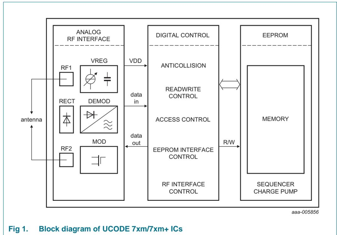
Fig 1. Block diagram of UCODE 7xm/7xm+ ICs
