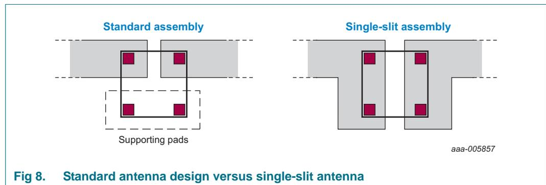
Fig 8. Standard antenna design versus single-slit antenna
