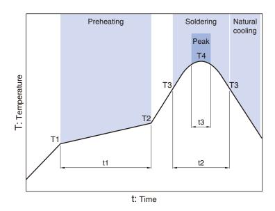
Soldering Preheating Peak Temp. Temp. Time Time Temp. Time T1 T2 T4 Т3 t3 150°C 180°C 60 to 120s 230°C 250°C 30s 5s
