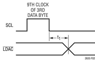
Figure 2b. LTC2635  $\overline{\text{LDAC}}$  Timing (QFN Package Only)
