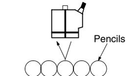
Sensing of small holes, narrow openings, or unevenness.
