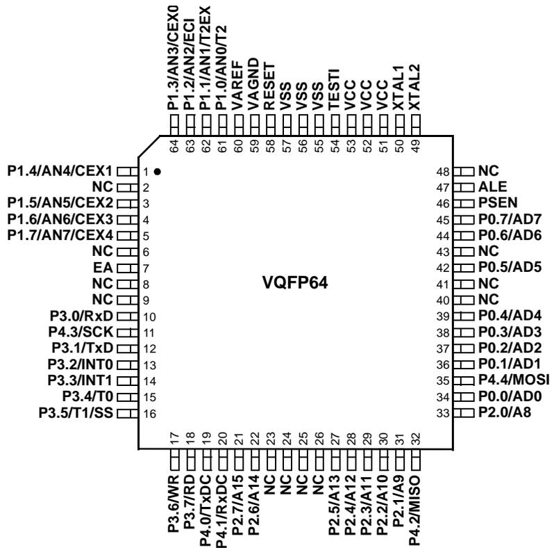
TESTI must be connected to VSS
