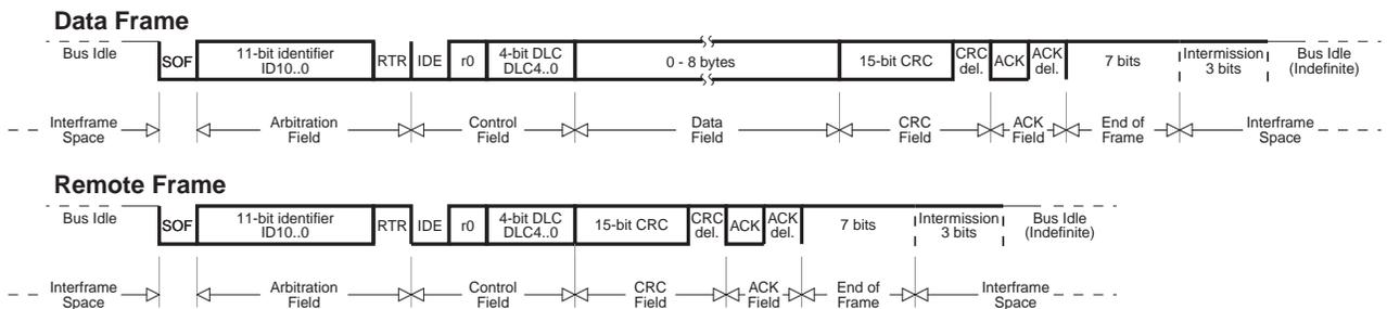
A message in the CAN standard frame format begins with the "Start Of Frame (SOF)", this is followed by the "Arbitration field" which consist of the identifier and the "Remote Transmission Request (RTR)" bit used to distinguish between the data frame and the data request frame called remote frame. The following "Control field" contains the "Identifier Extension (IDE)" bit and the "Data Length Code (DLC)" used to indicate the
