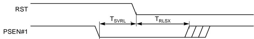
**Figure 83.** Flash Memory – Internal Busy Waveforms
