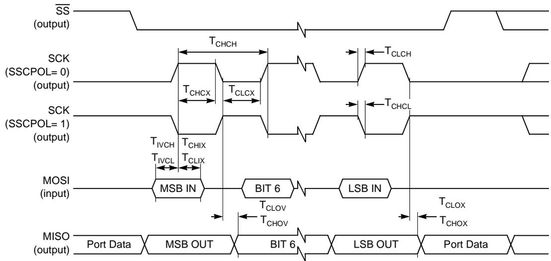
Note: 1.  $\overline{SS}$  handled by software using general purpose port pin.
