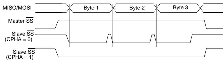
As shown in Figure 60, the first SCK edge is the MSB capture strobe. Therefore, the Slave must begin driving its data before the first SCK edge, and a falling edge on the  $\overline{SS}$  pin is used to start the transmission. The  $\overline{SS}$  pin must be toggled high and then low between each Byte transmitted (Figure 62).
