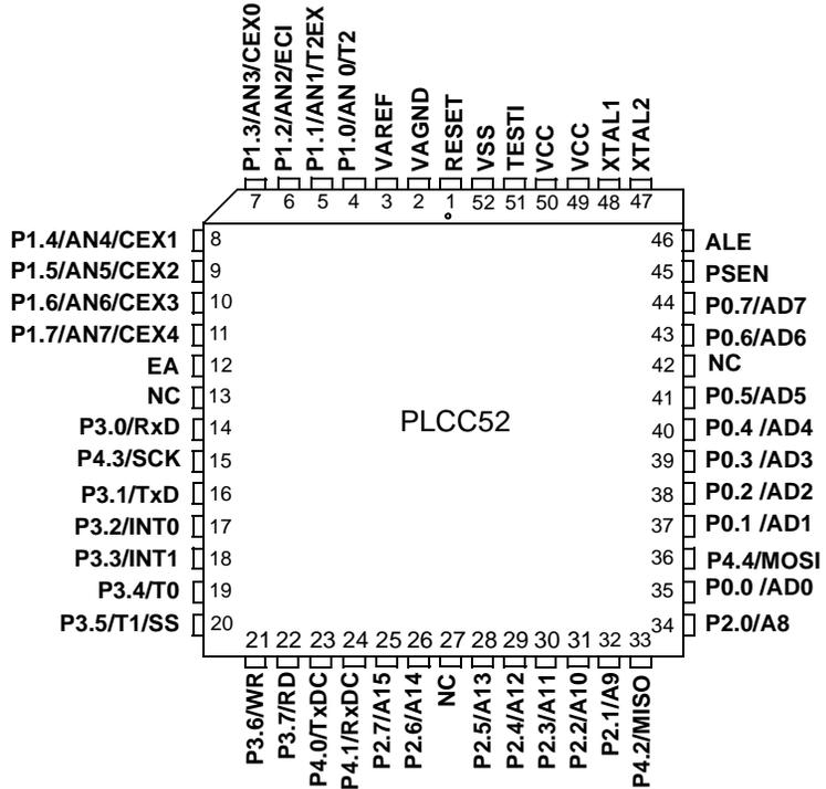
TESTI must be connected to VSS
