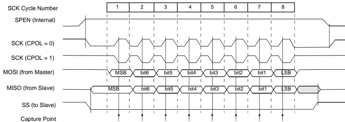
**Figure 61. Data Transmission Format (CPHA = 1)**
