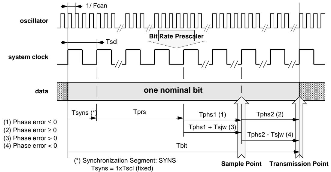
Tbit calculation:  $T_{bit} = T_{syns} + T_{prs} + T_{phs1} + T_{phs2}$
