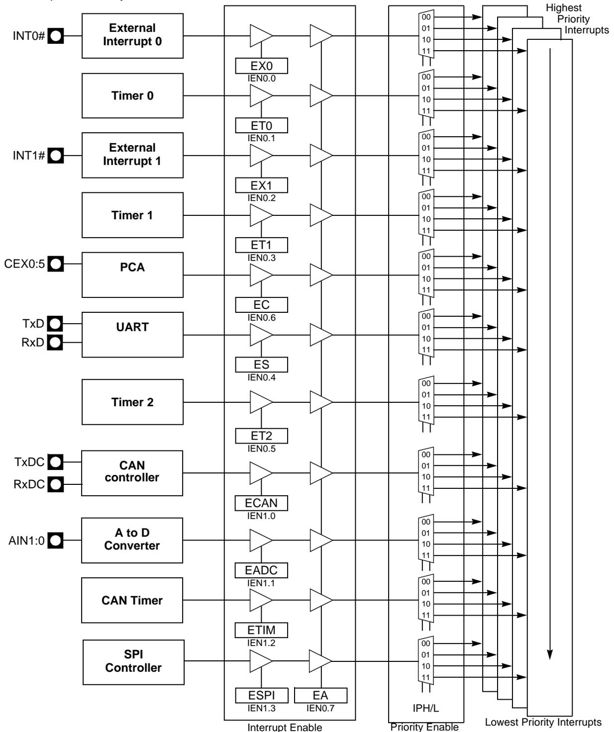
Each of the interrupt sources can be individually enabled or disabled by setting or clearing a bit in the Interrupt Enable register. This register also contains a global disable bit which must be cleared to disable all the interrupts at the same time.
