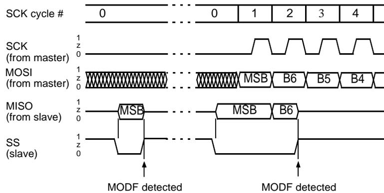
Note: when SS is discarded (SS disabled) it is not possible to detect a MODF error in slave mode because the SPI is internally selected. Also the SS pin becomes a general purpose I/O.
