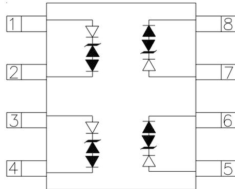
**Low Capacitance Protection of Two Differential Line Pairs**
