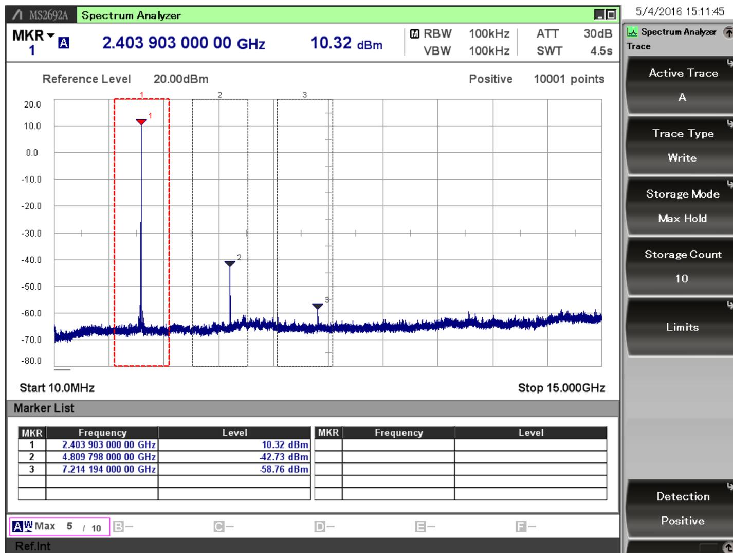
Figure 7.2. Typical Output Spectrum of the BRD4251B
