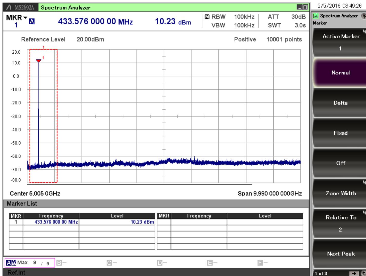
Figure 7.1. Typical Output Spectrum of the BRD4251B
