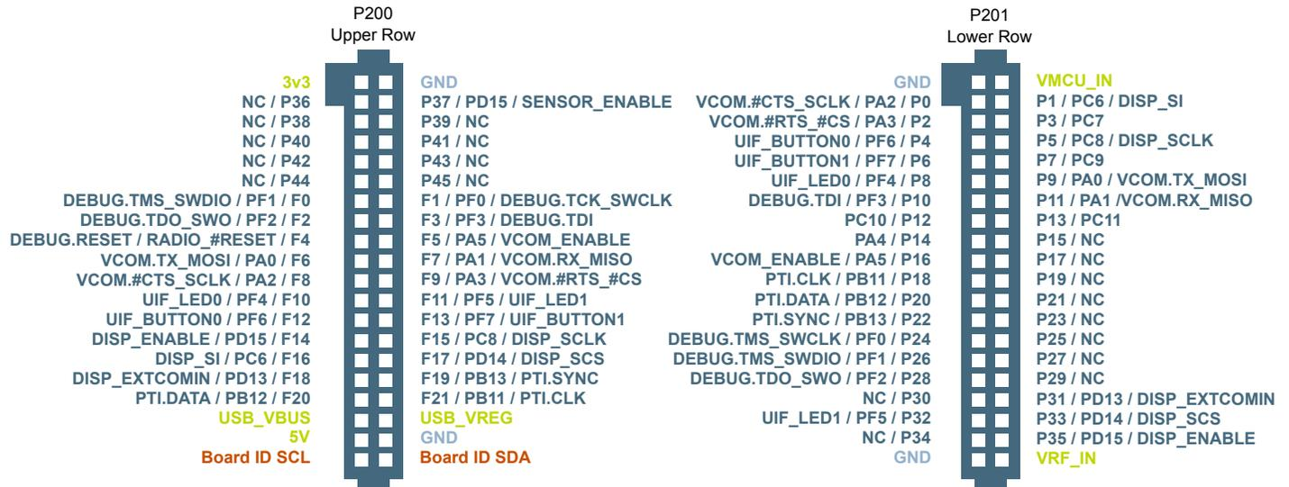
Figure 2.1. BRD4251B Radio Board Connector Pin Mapping
