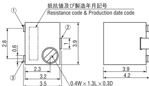
Unless otherwise specified, tolerance :  $\pm 0.3$  (Unit : mm)
