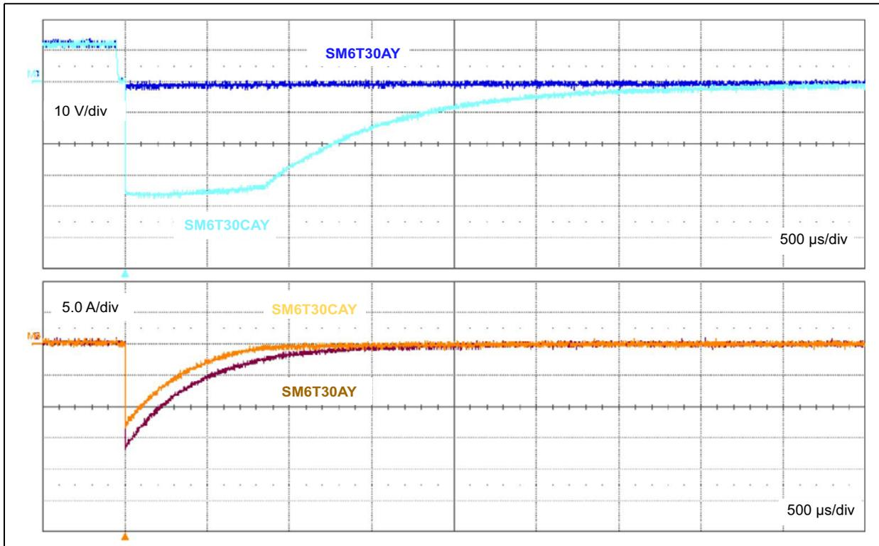
Figure 7. ISO 7637-2 pulse 2a response ( $V_S = 112\text{ V}$ )
