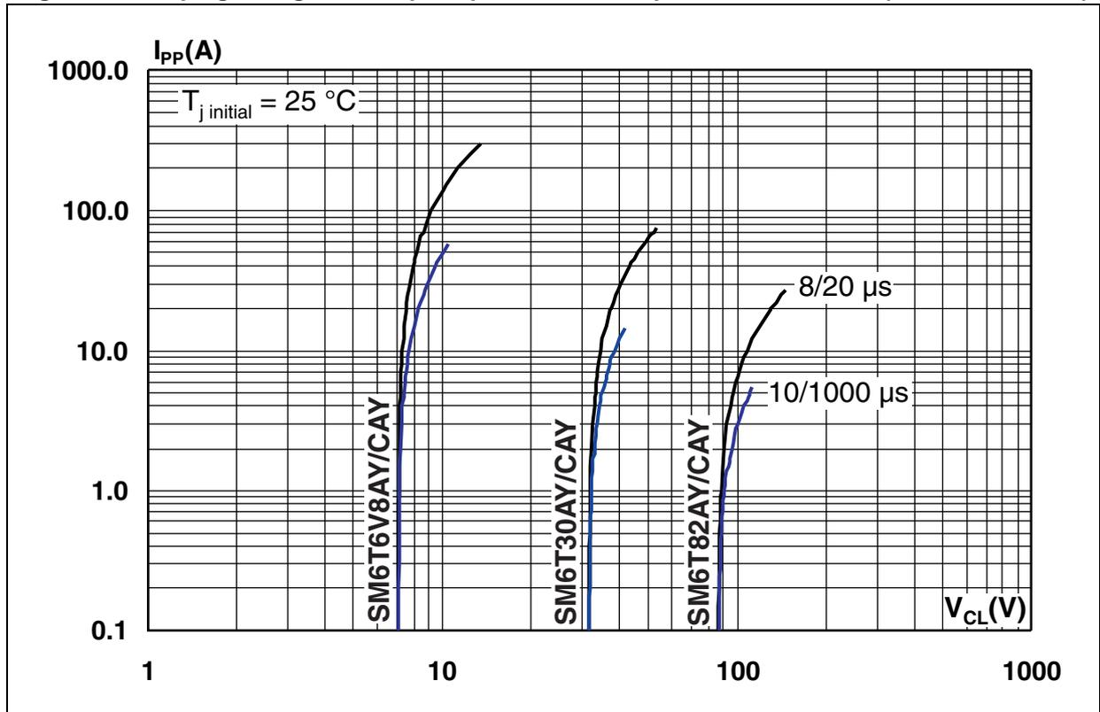
Figure 6. ISO 7637-2 pulse 1 response ( $V_S = -150\text{ V}$ )
