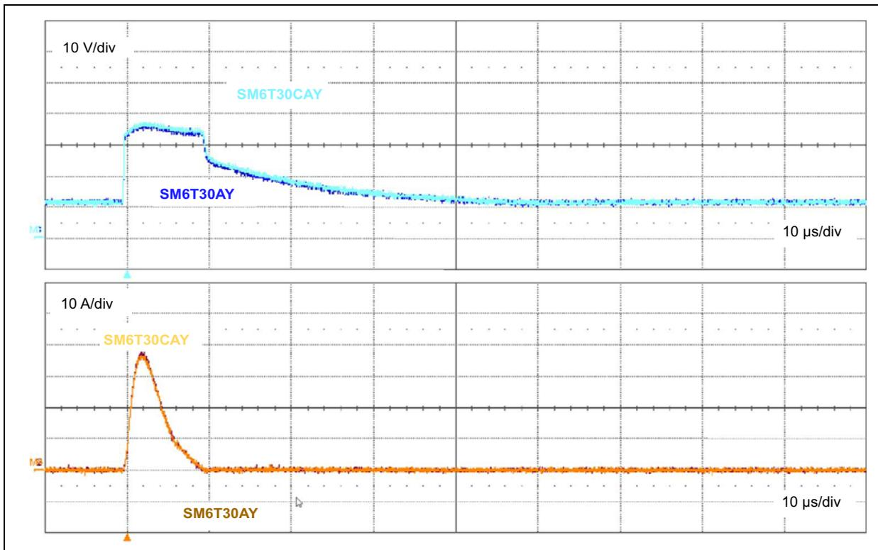
Figure 8. ISO 7637-2 pulse 3a response ( $V_S = -220\text{ V}$ )
