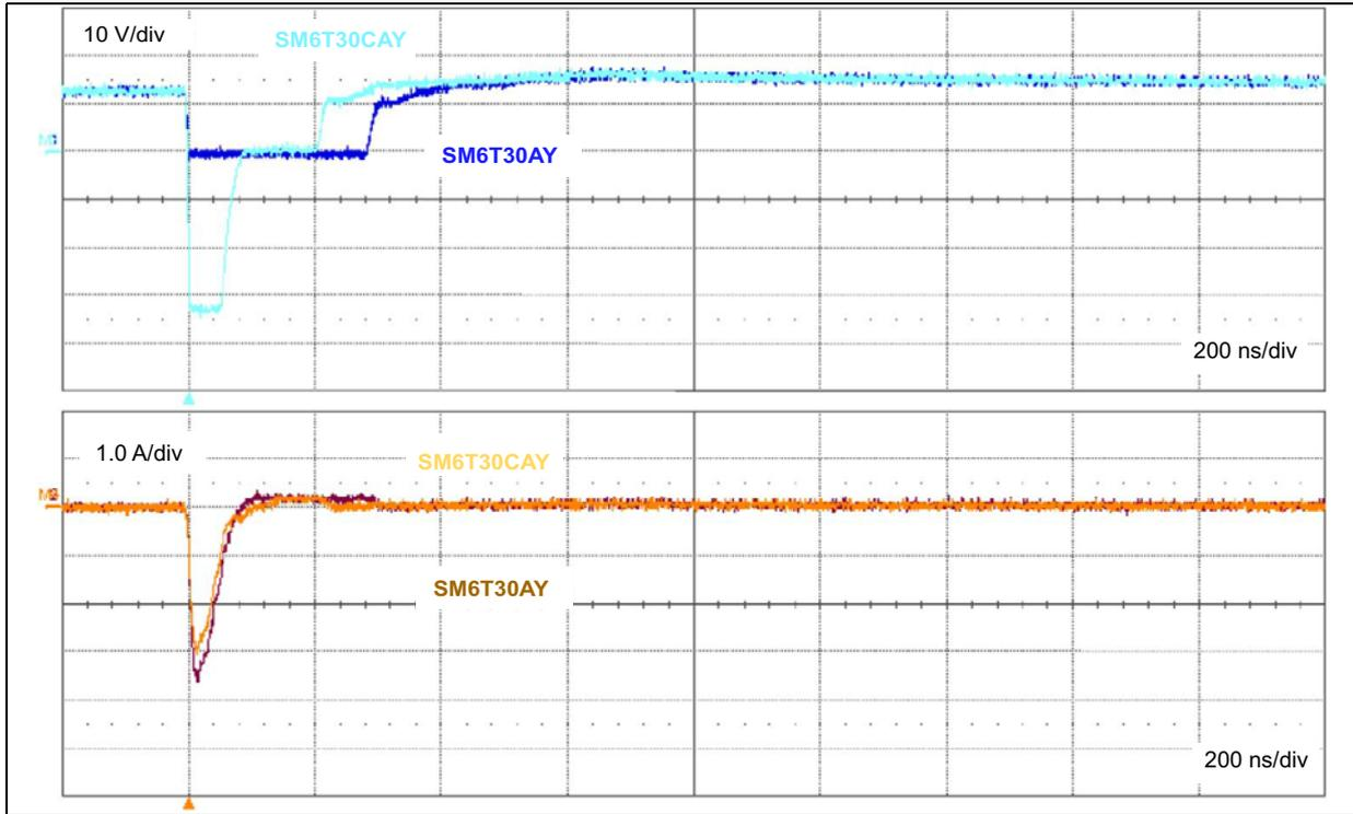
Figure 9. ISO 7637-2 pulse 3b response ( $V_S = 150\text{ V}$ )
