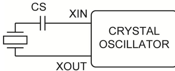
Figure 4. Crystal CL Value is Smaller than Oscillator CL Value
