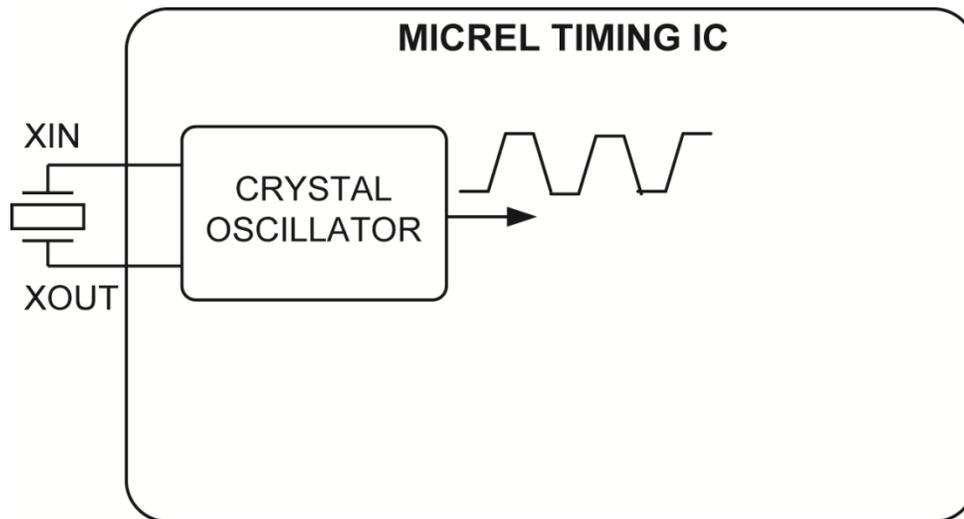
Figure 1. Example of Using a Crystal in a Micrel IC
