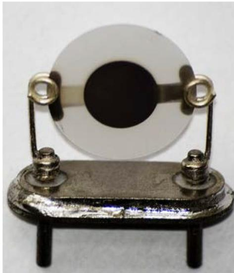
**Figure 2. Traditional Construction of a Quartz Crystal**
