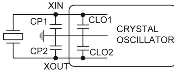
Figure 5. Crystal CL Value is Larger than Oscillator CL Value
