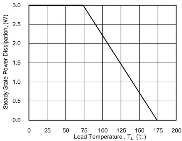
Fig. 2 - Steady State Power Derating Curve
