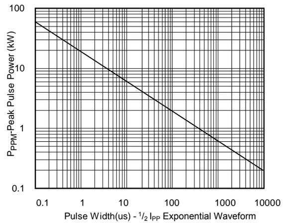
Fig. 3 - Peak Pulse Power Rating Curve
