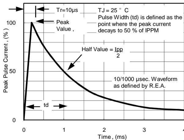
Fig. 4 - Pulse Waveform
