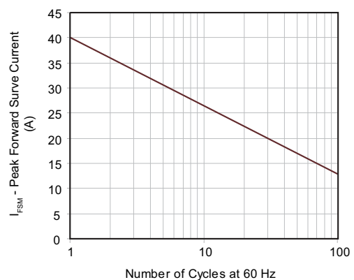
Figure 6 - Maximum Non-Repetitive Forward Surge Current Uni-Directional Only
