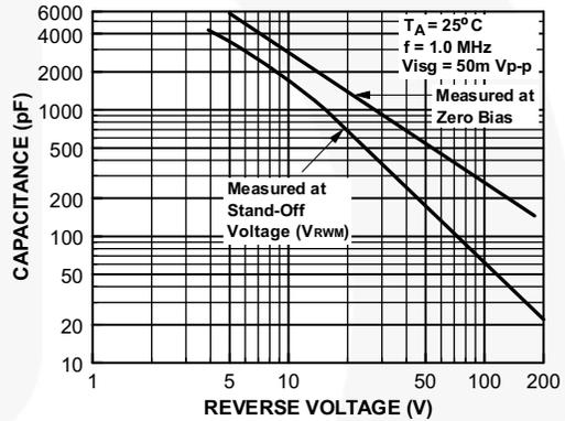
Figure 4. Junction Capacitance
