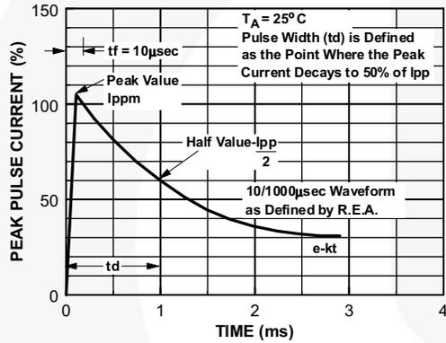
Figure 3. Pulse Waveform
