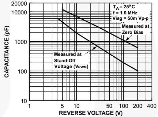
Figure 4. Junction Capacitance
