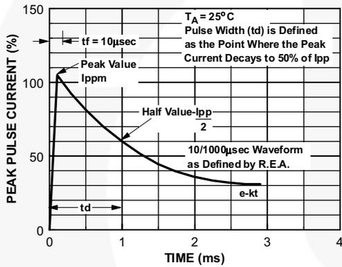
Figure 3. Pulse Waveform
