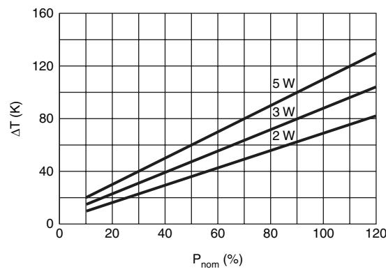
The temperature rise at the solder spot as a function of dissipated power
