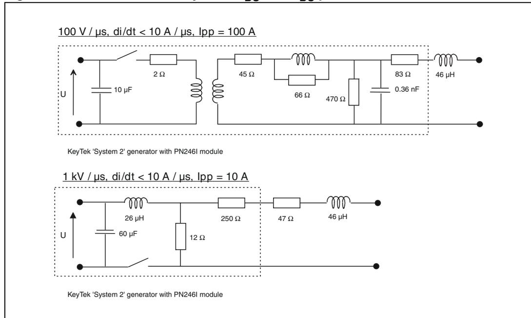
Figure 16. Test circuit 2 for  $I_{BO}$  and  $V_{BO}$  parameters
