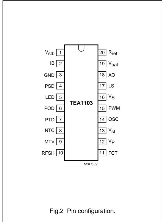
Fig.2 Pin configuration.
