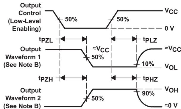
**Figure 5. Enable and Disable Times for 3-State Outputs**
