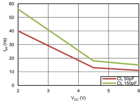
**Figure 1. Propagation Delay**
