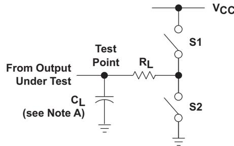
**Figure 2. Load Circuit**
