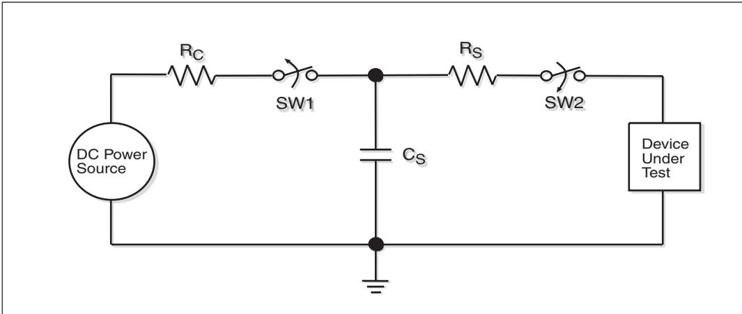
*Figure 7. ESD Test Circuit for Human Body Model*
