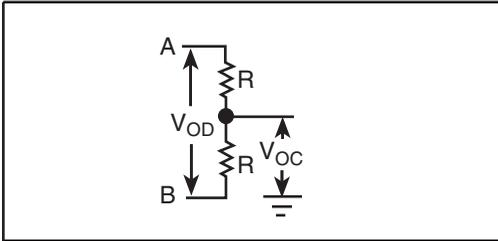
Figure 1. RS-485 Driver DC Test Load Circuit
