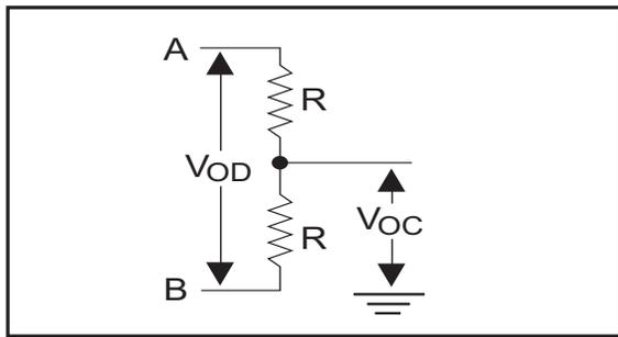
Figure 1. RS-485 Driver DC Test Load Circuit
