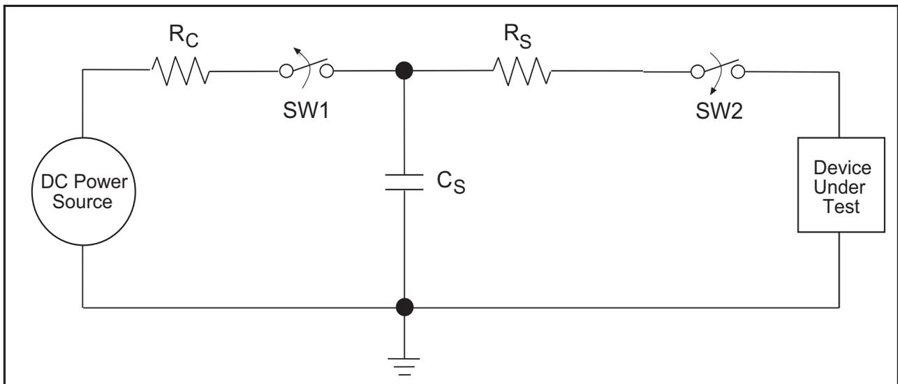
Figure 9. ESD Test Circuit for Human Body Model
