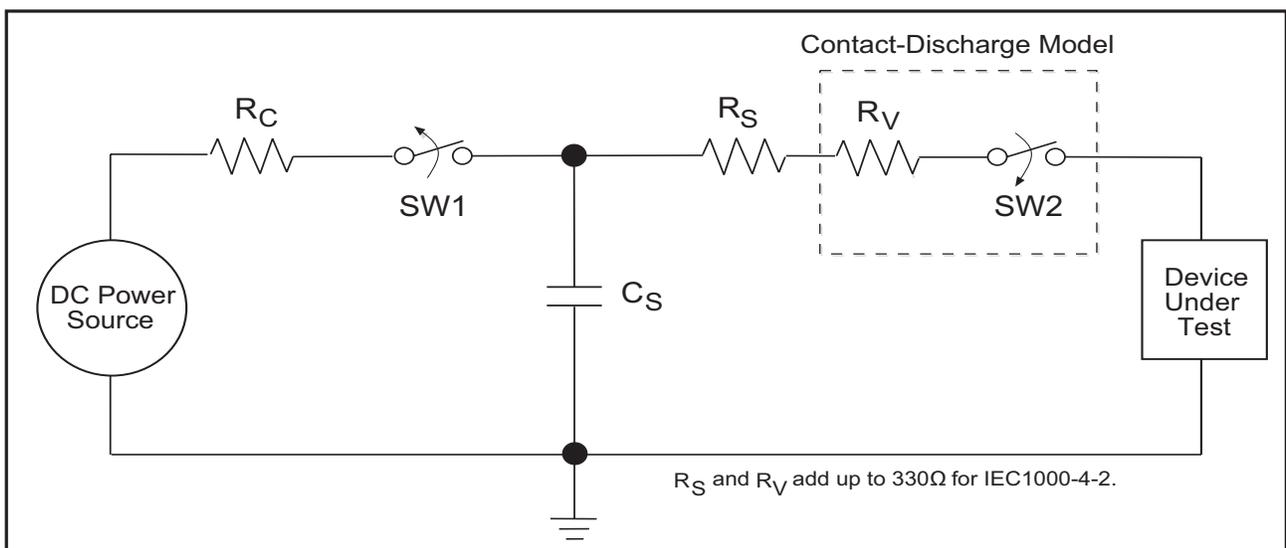
Figure 10. ESD Test Circuit for IEC1000-4-2
