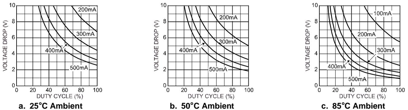
Figure 4. MIC5216-x.xBMM (MSOP-8) on 1-inch<sup>2</sup> Copper Cladding
