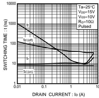
Fig.2 Switching Characteristics
