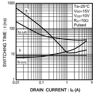
Fig.2 Switching Characteristics
