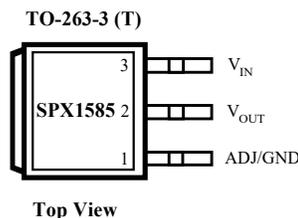
Note that TAB is connected to VOUT.
