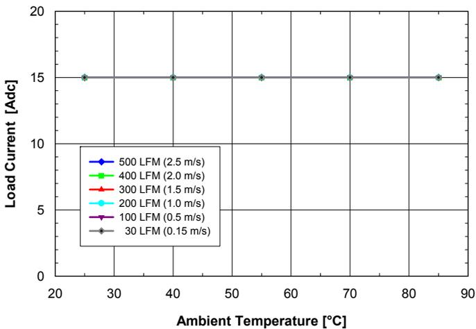
**Fig. 1.2V.3:** Available load current vs. ambient temperature and airflow rates for **SQ24S15012** converter mounted vertically with  $V_{in} = 24V$ , air flowing from pin 3 to pin 1 and maximum FET temperature  $\leq 120^{\circ}C$ .
