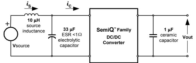
**Fig. 1.5V.14:** Test setup for measuring input reflected ripple currents,  $i_c$  and  $i_s$ .
