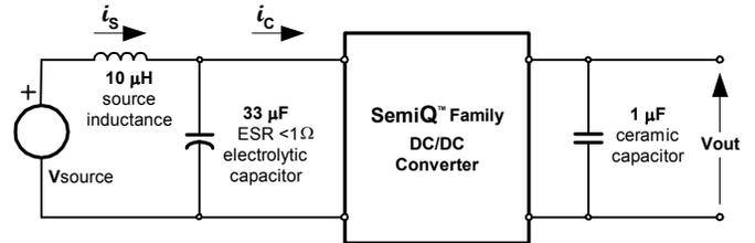
**Fig. 6.0V.14:** Test setup for measuring input reflected ripple currents,  $i_c$  and  $i_s$ .
