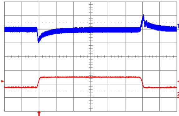
**Fig. 2.0V.11:** Output voltage response to load current step-change (3.75A – 7.5A – 3.75A) at  $V_{in} = 24V$ . Top trace: output voltage (100 mV/div.). Bottom trace: load current (5 A/div.). Current slew rate: 0.1 A/µs.  $C_o = 1 \mu F$  ceramic. Time scale: 0.2 ms/div.
