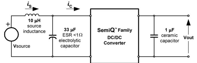
**Fig. 2.0V.14:** Test setup for measuring input reflected ripple currents,  $i_c$  and  $i_s$ .
