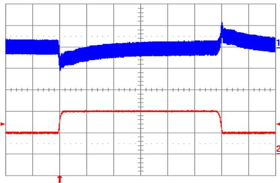
**Fig. 6.0V.11:** Output voltage response to load current step-change (2A – 4A – 2A) at  $V_{in} = 24V$ . Top trace: output voltage (100mV/div.). Bottom trace: load current (2A/div.). Current slew rate: 0.1 A/ $\mu s$ .  $C_o = 1 \mu F$  ceramic. Time scale: 0.2 ms/div.
