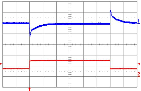
**Fig. 2.0V.12:** Output voltage response to load current step-change (3.75A – 7.5A – 3.75A) at  $V_{in} = 24V$ . Top trace: output voltage (100 mV/div.). Bottom trace: load current (5 A/div.). Current slew rate: 5 A/µs.  $C_o = 450 \mu F$  tantalum + 1 µF ceramic. Time scale: 0.2 ms/div.
