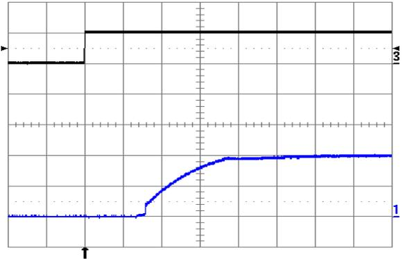
**Fig. 2.0V.10:** Turn-on transient at full rated load current (resistive) plus 10,000µF at  $V_{in} = 24V$ , triggered via ON/OFF pin. Top trace: ON/OFF signal (5 V/div.). Bottom trace: output voltage (1 V/div.). Time scale: 1 ms/div.
