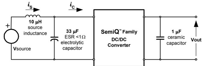
**Fig. 1.0V.14:** Test setup for measuring input reflected ripple currents,  $i_c$  and  $i_s$ .
