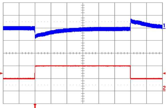
**Fig. 6.0V.12:** Output voltage response to load current step-change (2A – 4A – 2A) at  $V_{in} = 24V$ . Top trace: output voltage (100mV/div.). Bottom trace: load current (2A/div.). Current slew rate: 5 A/ $\mu s$ .  $C_o = 450 \mu F$  tantalum + 1  $\mu F$  ceramic. Time scale: 0.2 ms/div.
