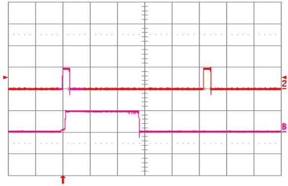
**Fig. 1.5V.18:** Load current (top trace, 20 A/div., 20 ms/div.) into a 10 mΩ short circuit during restart, at V<sub>in</sub> = 24V. Bottom trace (20 A/div., 2 ms/div.) is an expansion of the on-time portion of the top trace.
