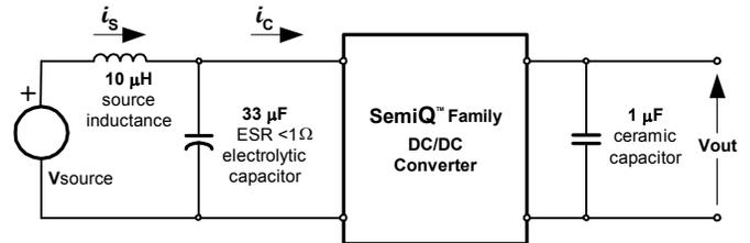
**Fig. 5.0V.14:** Test setup for measuring input reflected ripple currents,  $i_c$  and  $i_s$ .
