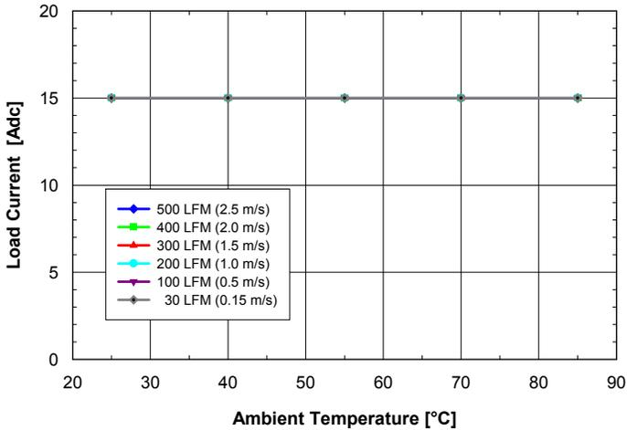
**Fig. 1.2V.1:** Available load current vs. ambient air temperature and airflow rates for **SQ24T15012** converter with **B** height pins mounted vertically with  $V_{in} = 24V$ , air flowing from pin 3 to pin 1 and maximum FET temperature  $\leq 120^{\circ}C$ .
