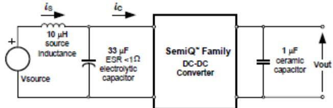
**Fig. 2.5V.16:** Input reflected ripple current,  $i_s$  (10 mA/div.), measured through 10  $\mu$ H at the source at
