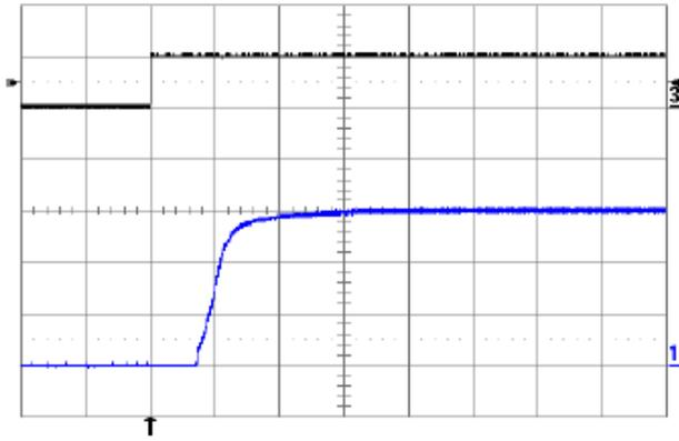
**Fig. 6.0V.11:** Output voltage response to load current step-change (2 A – 4 A – 2 A) at  $V_{in} = 48V$ . Top trace: output voltage (100 mV/div.). Bottom trace: load current (2 A/div.). Current slew rate:  $0.1A/\mu s$ .  $C_o = 1\mu F$  ceramic. Time scale: 0.2 ms/div.
