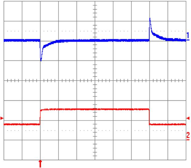
**Fig. 2.0V.13:** Output voltage ripple (20 mV/div.) at full rated load current into a resistive load with  $C_o = 10 \mu$ F tantalum + 1  $\mu$ F ceramic and  $V_{in} = 48$  V. Time scale: 1  $\mu$ s/div.
