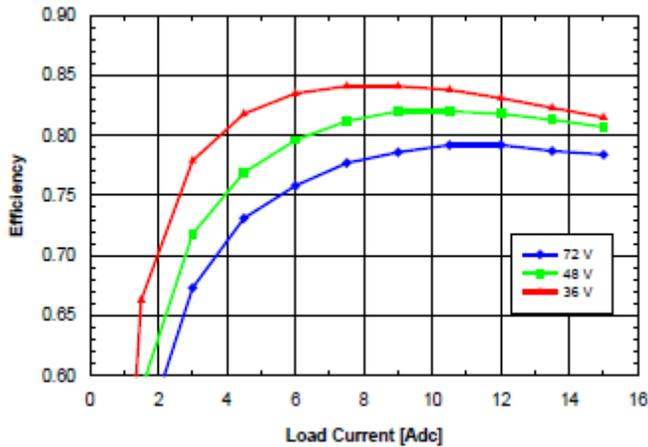
**Fig. 1.0V.6:** Efficiency vs. load current and ambient temperature for SQ48T/S15010 converter mounted vertically with  $V_{in} = 48\text{ V}$  and air flowing from pin 3 to pin 1 at a rate of 200 LFM (1.0 m/s).
