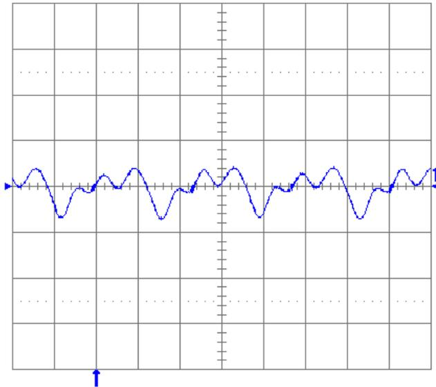
**Fig. 2.0V.13:** Output voltage ripple (20 mV/div.) at full ripple currents,  $i_c$  and  $i_s$
