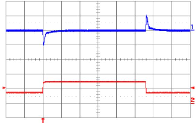
**Fig. 1.0V.13:** Output voltage ripple (20 mV/div.) at full rated load current into a resistive load with  $C_o = 10 \mu$ F tantalum + 1  $\mu$ F ceramic and  $V_{in} = 48$  V. Time scale: 1  $\mu$ s/div.
