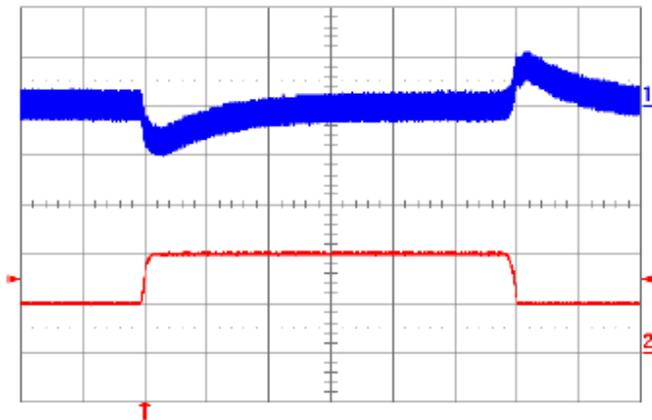
**Fig. 6.0V.13:** Output voltage ripple (50mV/div.) at full rated load current into a resistive load with  $C_o = 10\mu F$  tantalum +  $1\mu F$  ceramic and  $V_{in} = 48V$ . Time scale:  $1\mu s$ /div.
