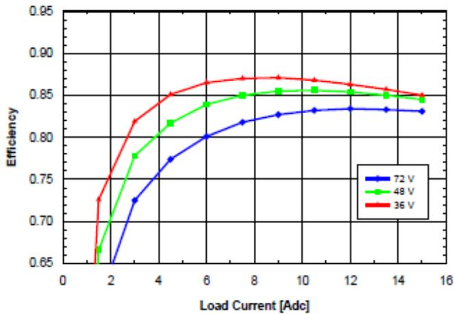
**Fig. 1.5V.6:** Efficiency vs. load current and ambient temperature for SQ48T/S15015 converter mounted vertically with  $V_{in} = 48\text{ V}$  and air flowing from pin 3 to pin 1 at a rate of 200 LFM (1.0 m/s).
