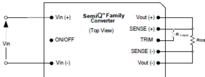
When trimming up, care must be taken not to exceed the converter's maximum allowable output power. See the previous section for a complete discussion of this requirement.
