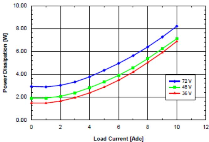
**Fig. 5.0V.8:** Power dissipation vs. load current and ambient temperature for SQ48T/S10050 converter mounted vertically with  $V_{in} = 48\text{V}$  and air flowing from pin 3 to pin 1 at a rate of 200 LFM (1.0m/s).
