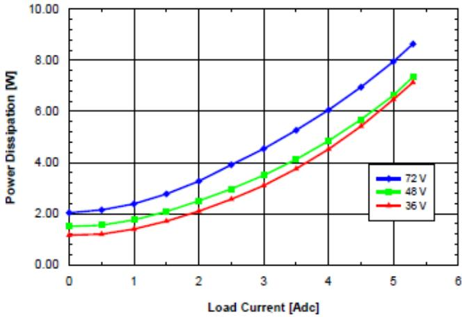
**Fig. 8.0V.8:** Power dissipation vs. load current and ambient temperature for SQ48T/S05080 converter mounted vertically with  $V_{in} = 48\text{V}$  and air flowing from pin 3 to pin 1 at a rate of 200 LFM (1.0 m/s).
