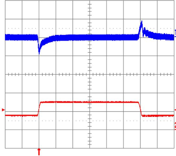
step-change (3.75 A – 7.5 A – 3.75 A) at  $V_{in} = 48$  V.
