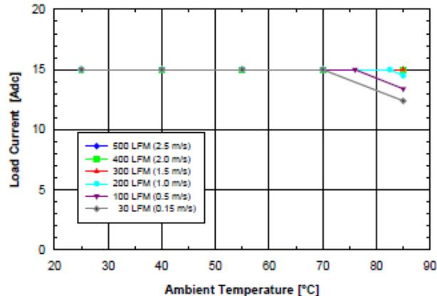
**Fig. 1.5V.2:** Available load current vs. ambient air temperature and airflow rates for SQ48T15015 converter with D height pins mounted horizontally with  $V_{in} = 48\text{ V}$ , air flowing from pin 3 to pin 1, and maximum FET temperature  $\leq 120\text{ }^\circ\text{C}$ .
