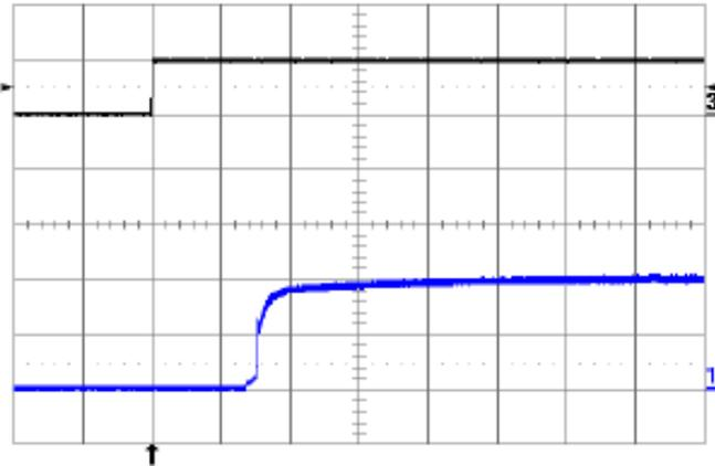
**Fig. 1.0V.10:** Turn-on transient at full rated load current (resistive) plus 10,000  $\mu\text{F}$  at  $V_{in} = 48\text{ V}$ , triggered via ON/OFF pin. Top trace: ON/OFF signal (5 V/div.). Bottom trace: output voltage (0.5 V/div.). Time scale: 2 ms/div.
