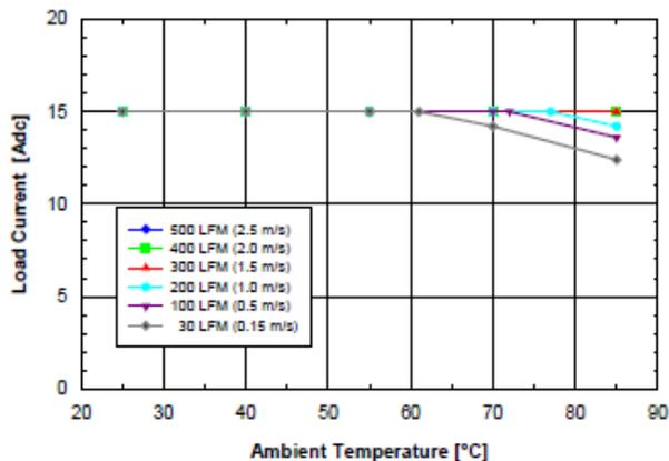
**Fig. 2.0V.4:** Available load current vs. ambient air
