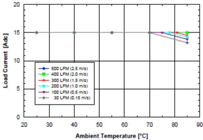
**Fig. 1.8V.4:** Available load current vs. ambient air temperature and airflow rates for SQ48S15018 converter mounted horizontally with  $V_{in} = 48\text{ V}$ , air flowing from pin 3 to pin 1, and maximum FET temperature  $\leq 120\text{ }^{\circ}\text{C}$ .
