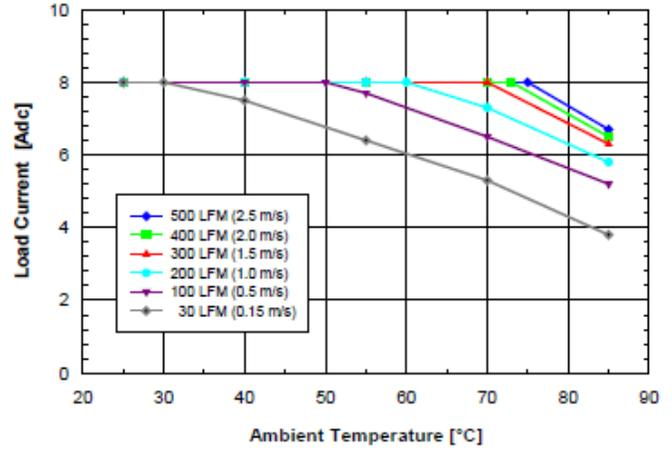
**Fig. 6.0V.4:** Available load current vs. ambient air temperature and airflow rates for SQ48S08060 converter mounted horizontally with  $V_{in} = 48V$ , air flowing from pin 3 to pin 1, and maximum FET temperature  $\leq 120^{\circ}C$ .
