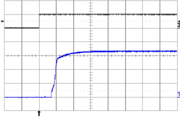
**Fig. 3.3V.10:** Turn-on transient at full rated load current (resistive) plus 10,000  $\mu\text{F}$  at  $V_{in} = 48\text{ V}$ , triggered via ON/OFF pin. Top trace: ON/OFF signal (5 V/div.). Bottom trace: output voltage (1 V/div.). Time scale: 2 ms/div.
