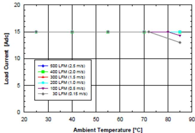
**Fig. 1.2V.2:** Available load current vs. ambient air temperature and airflow rates for SQ48T15012 converter with D height pins mounted horizontally with  $V_{in} = 48\text{ V}$ , air flowing from pin 3 to pin 1, and maximum FET temperature  $\leq 120\text{ }^\circ\text{C}$ .
