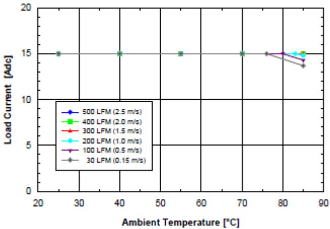
**Fig. 1.5V.4:** Available load current vs. ambient air temperature and airflow rates for SQ48S15015 converter mounted horizontally with  $V_{in} = 48\text{ V}$ , air flowing from pin 3 to pin 1, and maximum FET temperature  $\leq 120\text{ }^{\circ}\text{C}$ .
