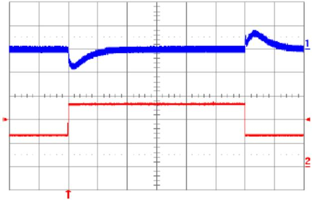
**Fig. 8.0V.13:** Output voltage ripple (50 mV/div.) at full rated load current into a resistive load with  $C_o = 10 \mu F$  tantalum +  $1\mu F$  ceramic and  $V_{in} = 48V$ . Time scale: 1 $\mu$ s/div.
