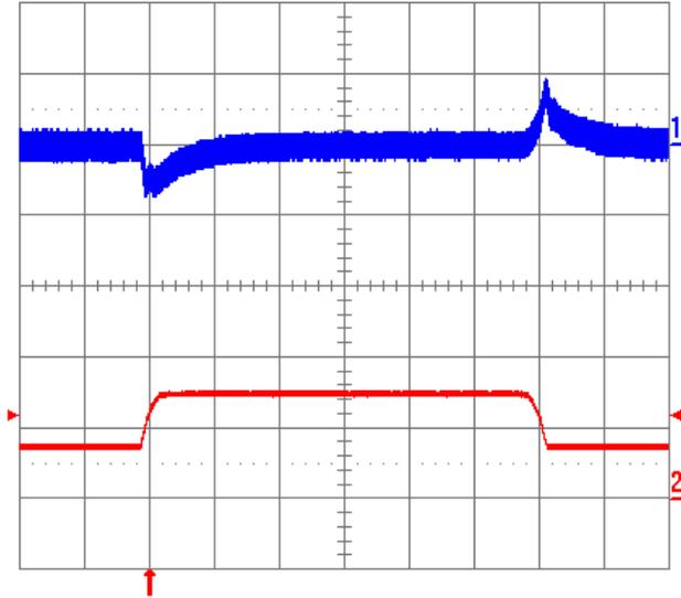
**Fig. 3.3V.13:** Output voltage ripple (20 mV/div.) at full rated load current into a resistive load with  $C_o = 10 \mu\text{F}$  tantalum +  $1 \mu\text{F}$  ceramic and  $V_{in} = 48 \text{ V}$ . Time scale:  $1 \mu\text{s}/\text{div}$ .
