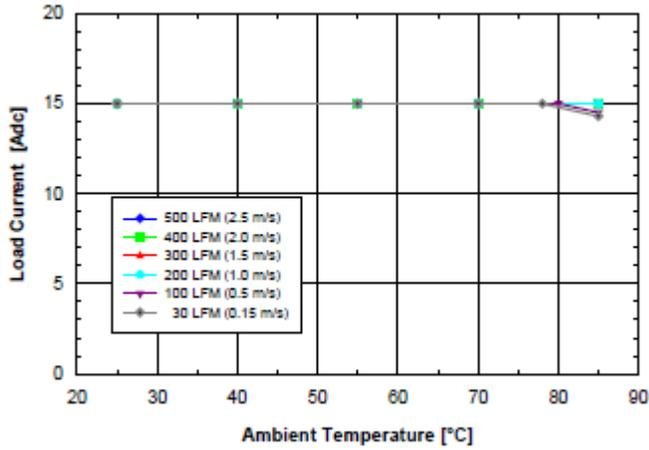
**Fig. 1.2V.4:** Available load current vs. ambient air temperature and airflow rates for SQ48S15012 converter mounted horizontally with  $V_{in} = 48\text{ V}$ , air flowing from pin 3 to pin 1, and maximum FET temperature  $\leq 120\text{ }^{\circ}\text{C}$ .
