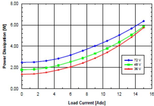
mounted vertically with  $V_{in} = 48\text{ V}$  and air flowing from pin 3 to pin 1 at a rate of 200 LFM (1.0 m/s).
