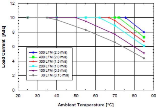
**Fig. 5.0V.2:** Available load current vs. ambient air temperature and airflow rates for SQ48T10050 converter with D height pins mounted horizontally with Vin = 48V, air flowing from pin 3 to pin 1, and maximum FET temperature ≤ 120°C.
