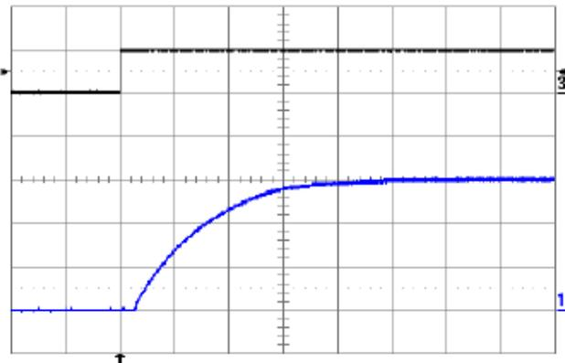
**Fig. 6.0V.12:** Output voltage response to load current step-change (2 A – 4 A – 2 A) at  $V_{in} = 48V$ . Top trace: output voltage (100 mV/div.). Bottom trace: load current (2 A/div.). Current slew rate:  $5A/\mu s$ .  $C_o = 450\mu F$  tantalum +  $1\mu F$  ceramic. Time scale: 0.2ms/div.
