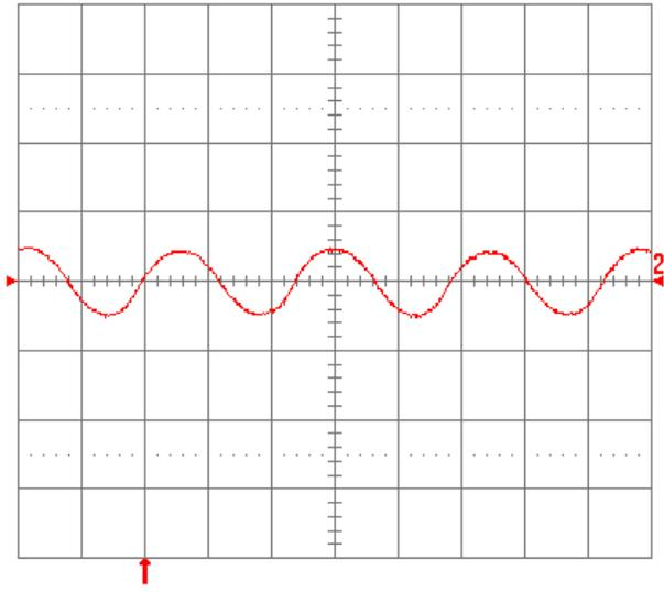
full rated load current and  $V_{in} = 48\text{ V}$ . Refer to Fig. 2.5V.14 for test setup. Time scale:  $1\ \mu\text{s}/\text{div}$ .
