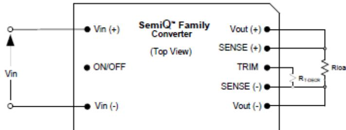
Trimming/sensing beyond 110% of the rated output voltage is not an acceptable design practice, as this condition could cause unwanted triggering of the output overvoltage protection (OVP) circuit. The designer should ensure that the difference between the voltages across the converter’s output pins and its sense pins does not exceed 10% of  $V_{OUT(NOM)}$ , or:
