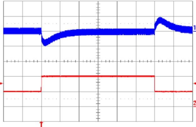
**Fig. 12V.13:** Output voltage ripple (50 mV/div.) at full rated load current into a resistive load with  $C_o = 10\mu F$  tantalum + 1  $\mu F$  ceramic and  $V_{in} = 48V$ . Time scale: 1 $\mu$ s/div.
