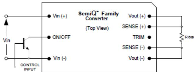
The positive logic version turns on when the ON/OFF pin is at a logic high and turns off when at a logic low. The converter is on when the ON/OFF pin is left open. See Electrical Specifications for logic high/low definitions.
