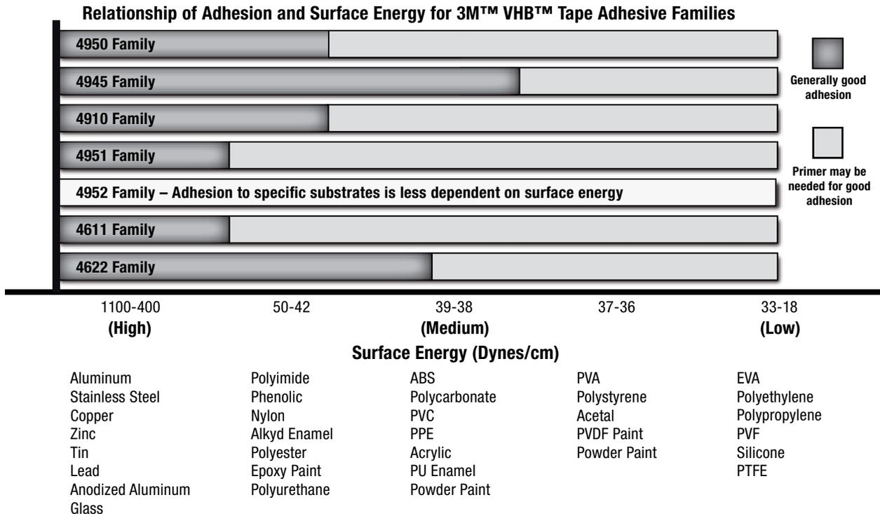
**NOTES:** There are a wide variety of formulations, surfaces finishes and surface treatments available on substrate materials which can affect adhesion. This chart is intended to provide only a rough estimate of the adhesion levels which can be expected on some common materials relative to a reference surface such as aluminum. Foam type can affect and/or limit maximum adhesive strength.
