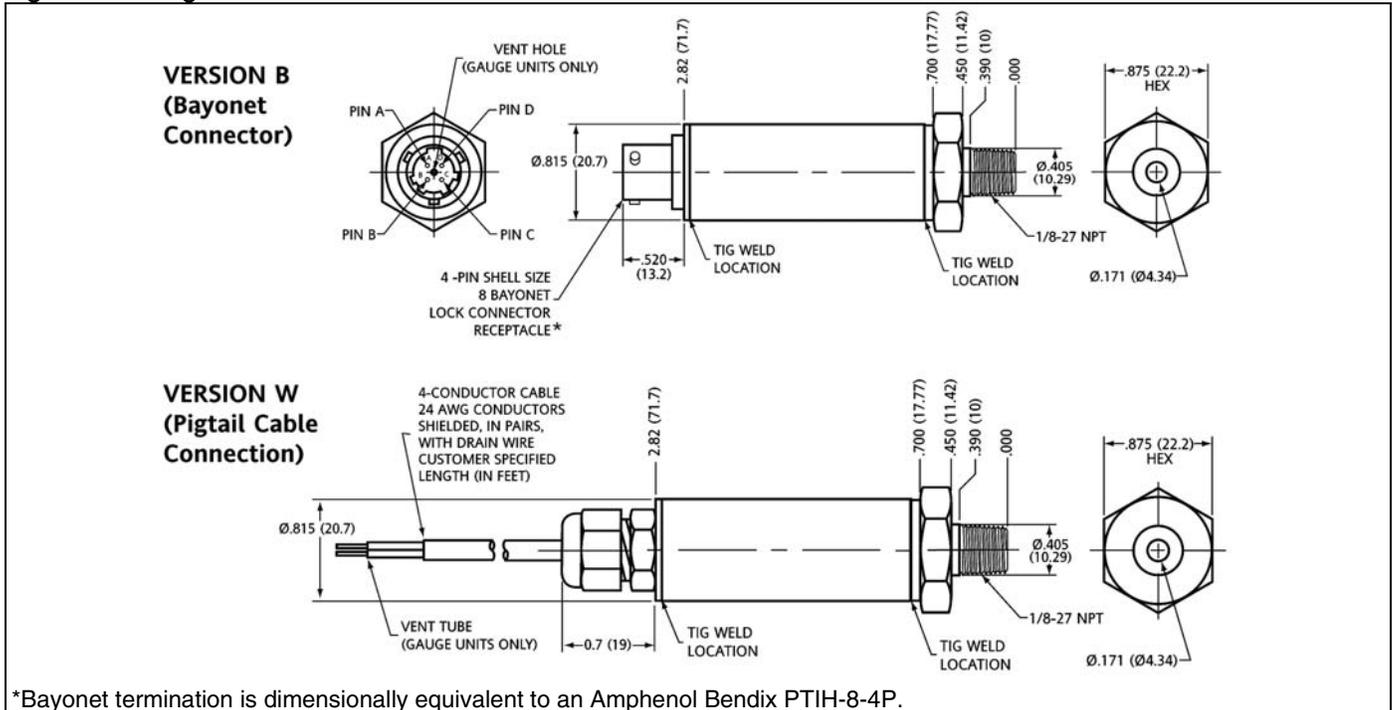
\*Bayonet termination is dimensionally equivalent to an Amphenol Bendix PTIH-8-4P.
