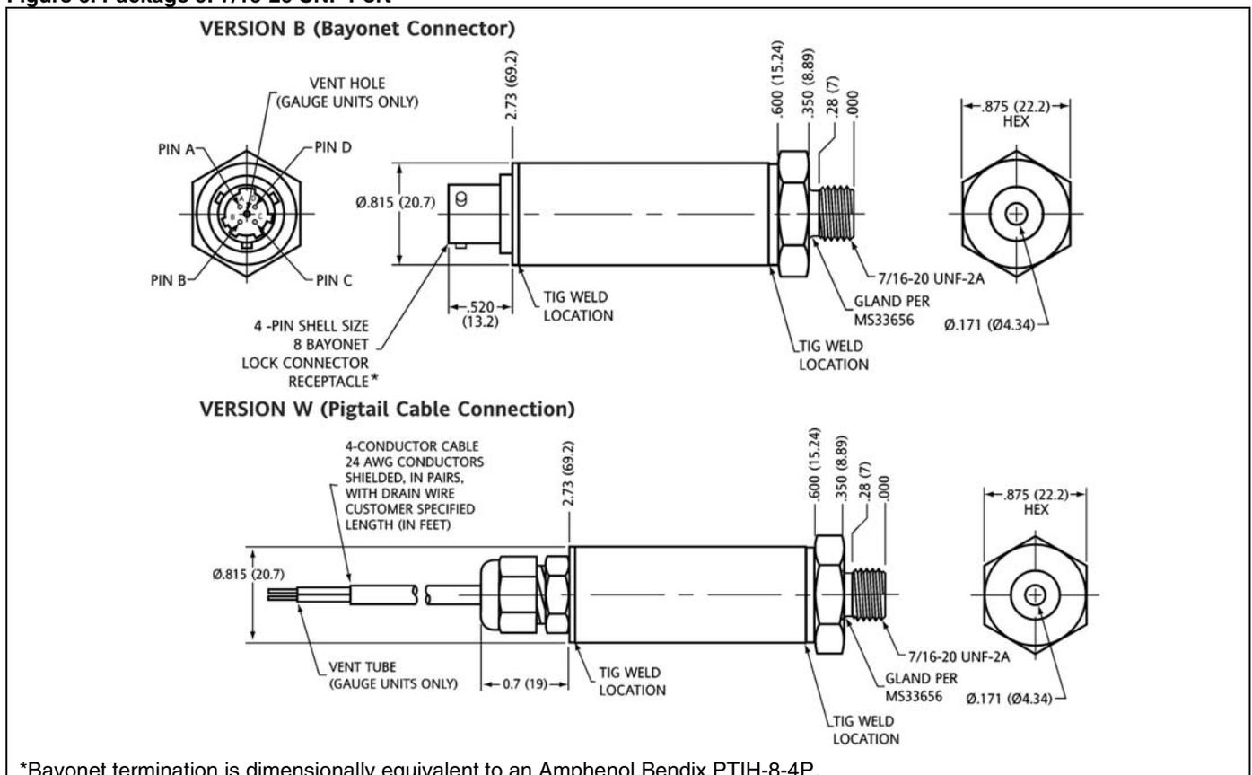
\*Bayonet termination is dimensionally equivalent to an Amphenol Bendix PTIH-8-4P.
