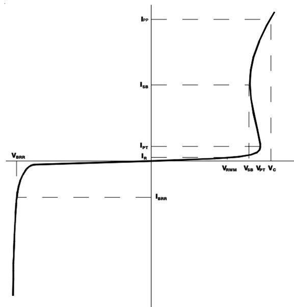
**Figure 4 - EPD TVS IV Characteristic Curve**
