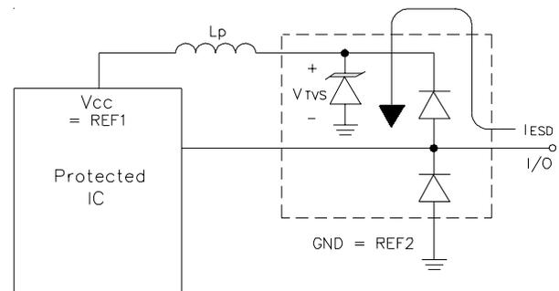
**Figure 3 - Rail-To-Rail Protection Using RailClamp TVS Arrays**
