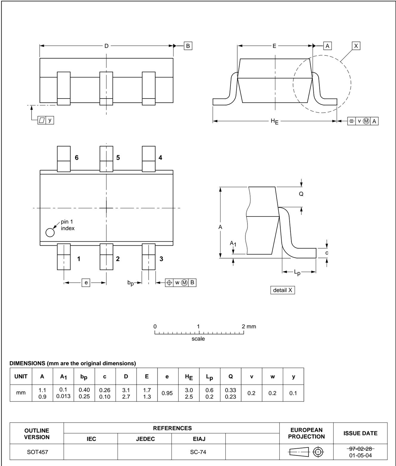
40 V low  $V_{CEsat}$  NPN/PNP transistor
