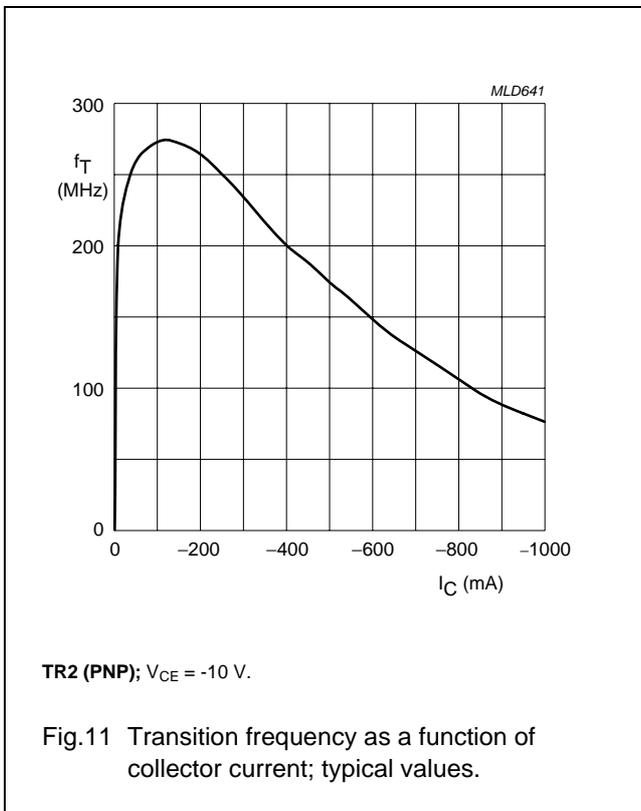
40 V low  $V_{CEsat}$  NPN/PNP transistor
