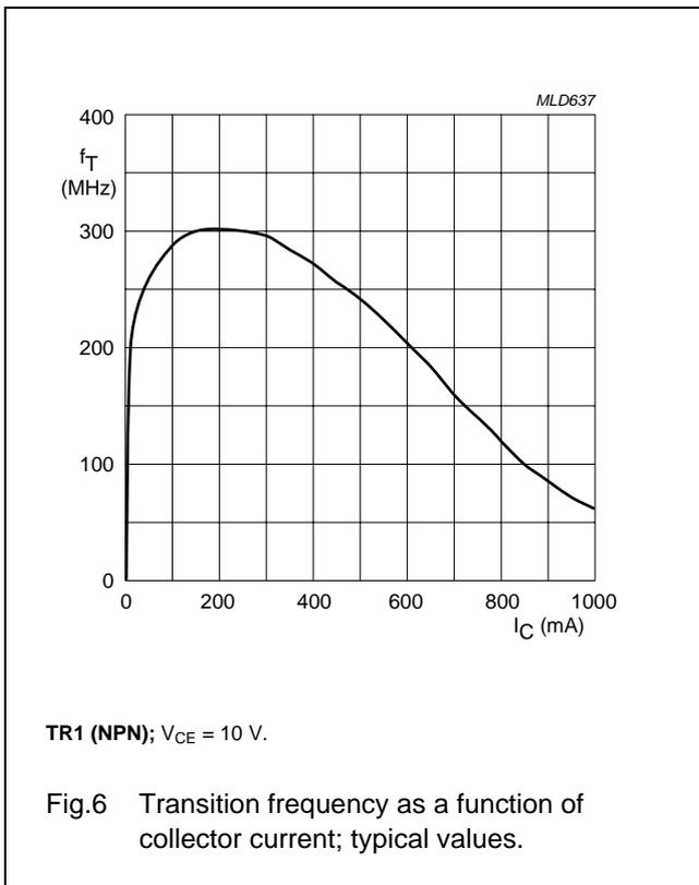
40 V low  $V_{CEsat}$  NPN/PNP transistor
