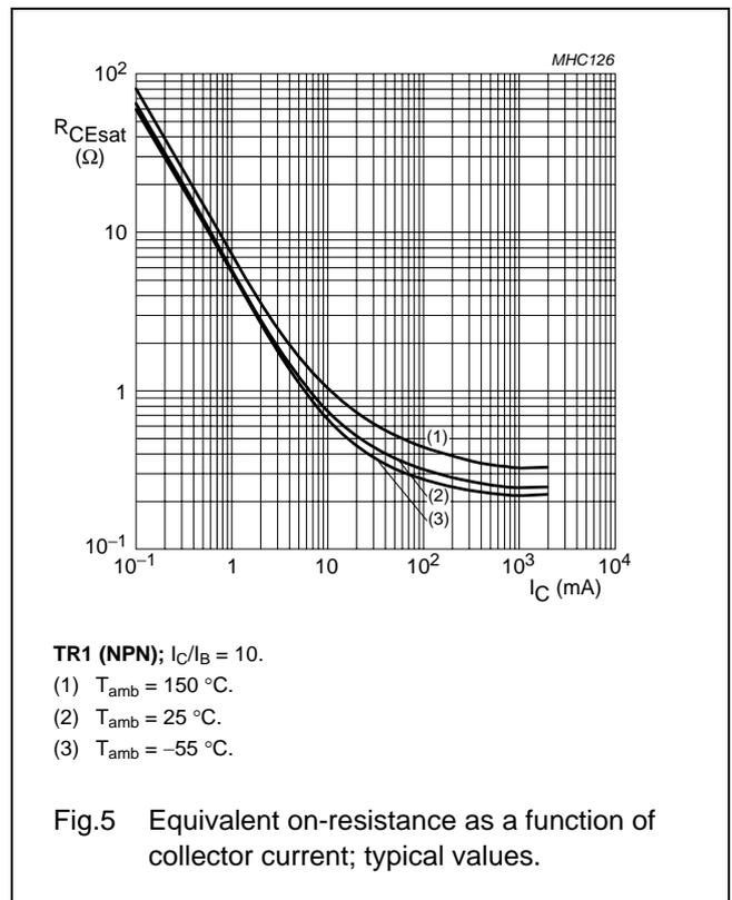
40 V low  $V_{CEsat}$  NPN/PNP transistor
