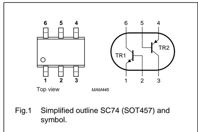
40 V low  $V_{CEsat}$  NPN/PNP transistor
