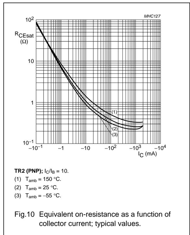
40 V low  $V_{CEsat}$  NPN/PNP transistor
