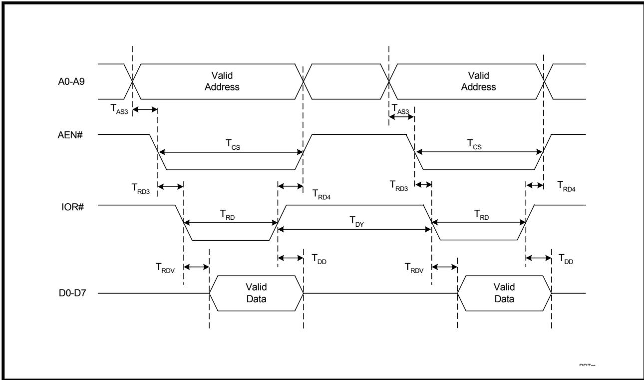
FIGURE 22. DATA BUS WRITE TIMING IN PC MODE
