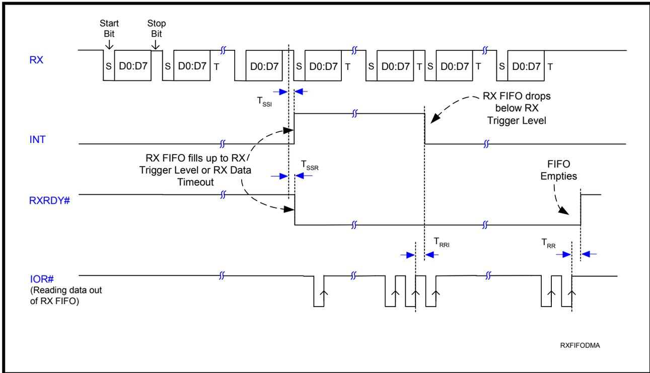
FIGURE 27. TRANSMIT READY & INTERRUPT TIMING [FIFO MODE, DMA MODE DISABLED]
