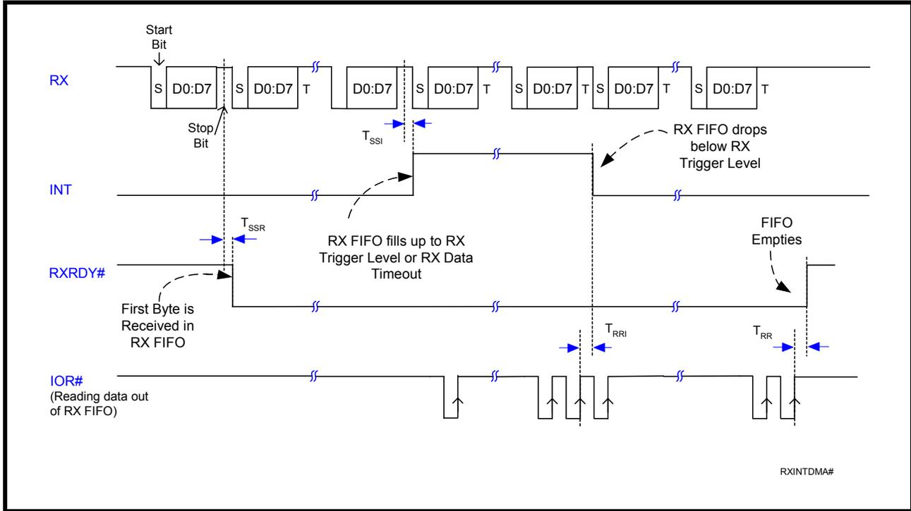
FIGURE 26. RECEIVE READY & INTERRUPT TIMING [FIFO MODE, DMA ENABLED]
