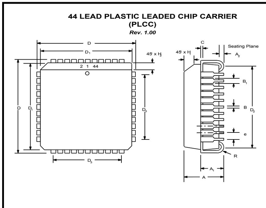
Note: The control dimension is the millimeter column
