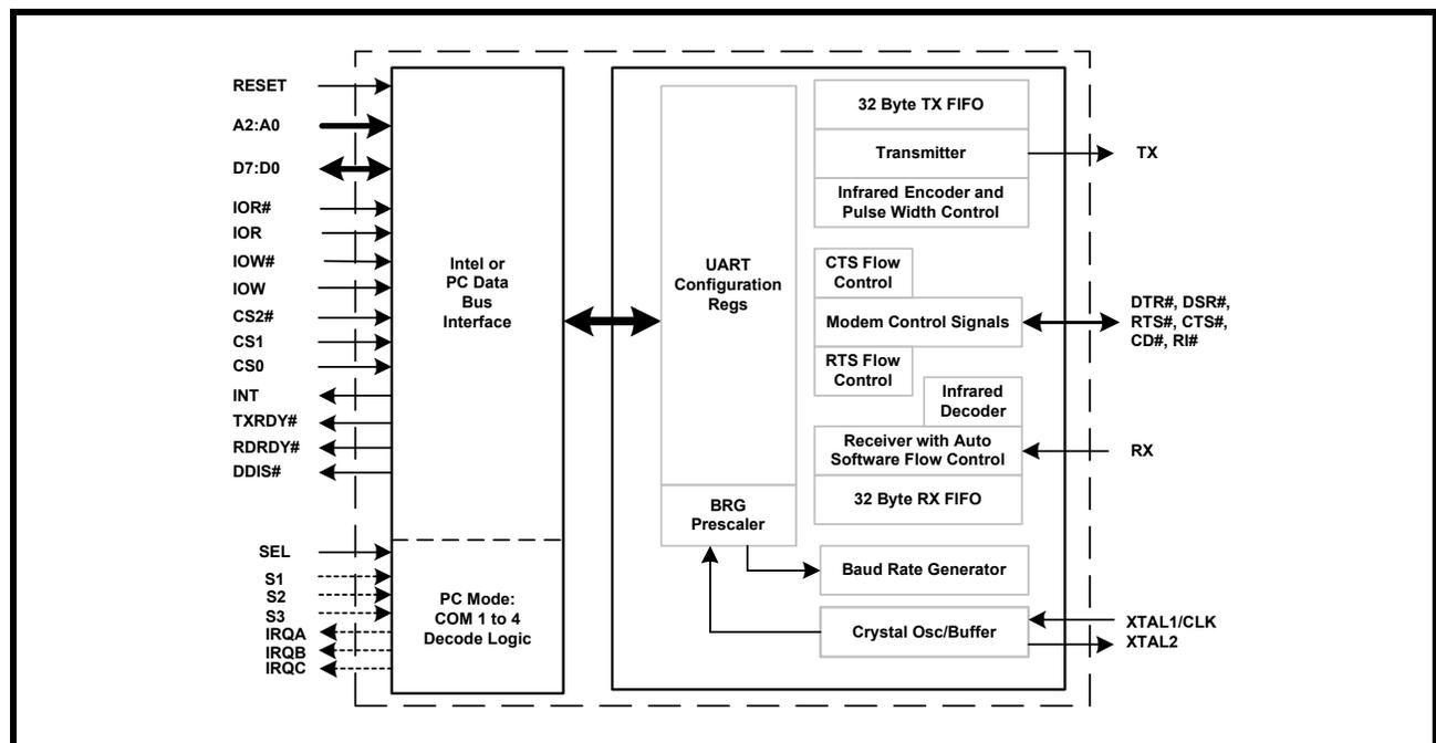
FIGURE 2. INTEL AND PC MODE PIN OUT
